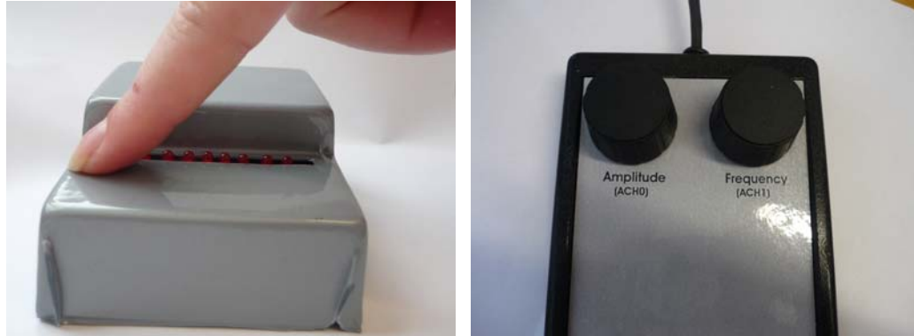
Figure 5.2 A-B (A) Running light box to train participant scanning speed. (B) 2-dial control box for adjusting vibratory frequency and amplitude.
