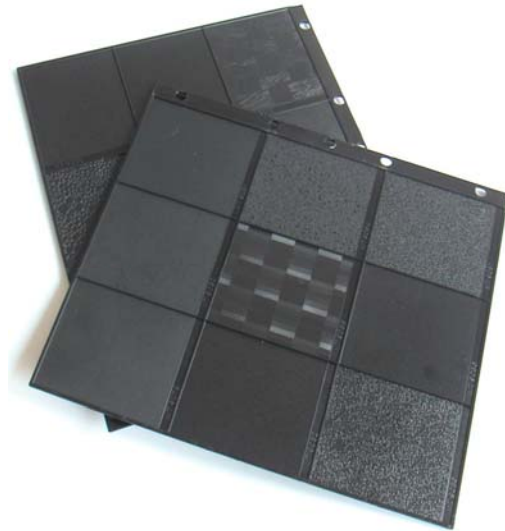
Figure 3.3.4. Standex mould decorations before cutting them into separate plaques.
