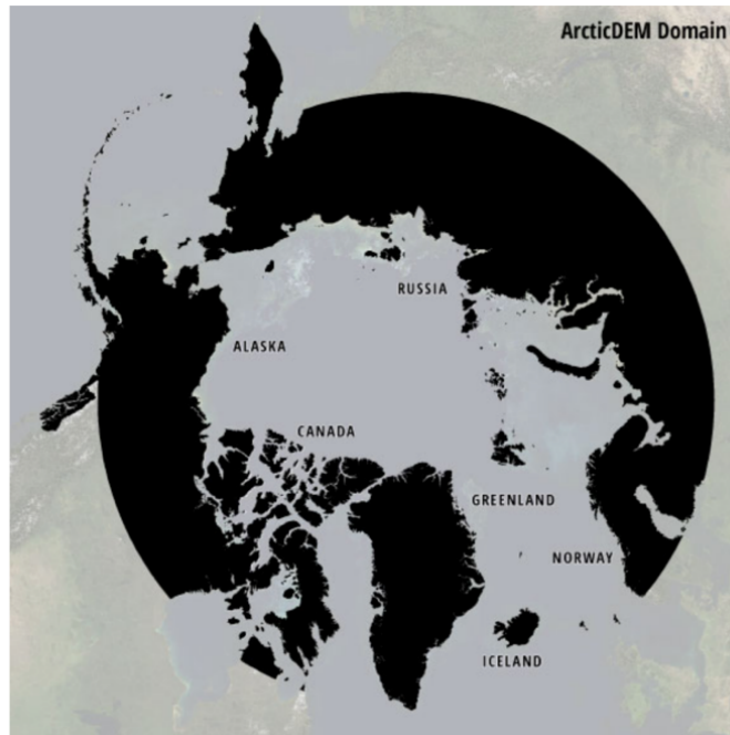
Figure 1.8 The ArcticDEM domain (black), including all land area north of 60° (Porter et al. 2018). Data were available in 50 x 50 km tiles at a 5 m resolution when I started my PhD and now at 2 m and 10 m resolutions. Data are freely available at https://www.pgc.umn.edu/data/arcticdem/ .
