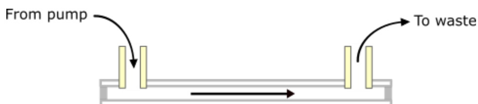
Figure 23. Flow cell flow dynamics of sample. Sample is infused into the flow cell through an inlet port (left). The sample then proceeds through the volume of the flow chamber. The sample exits through an opposite port (right). This method allows a sample to be interchanged without having to remove a microscope slide from the sample stage.
