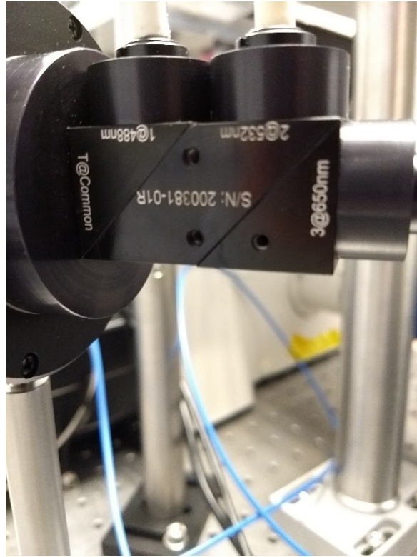
Figure 15. Combining lasers into a single output fibre. 488 and 633 nm laser paths were combined into the same single fibre using a laser combiner (OZ optics).
