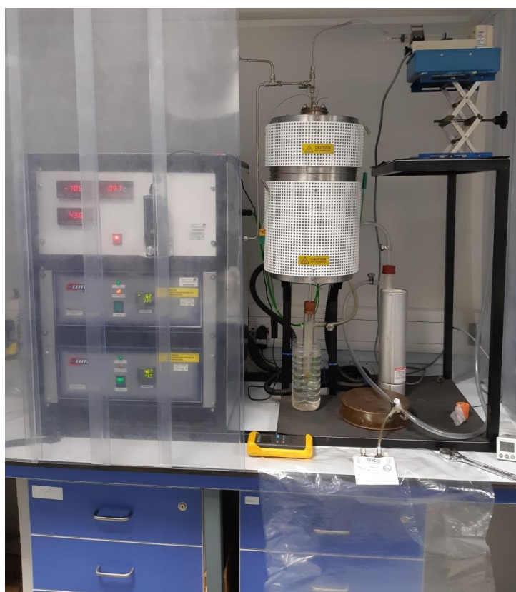
Figure 3.14 An image of the steam activation reactor set-up
