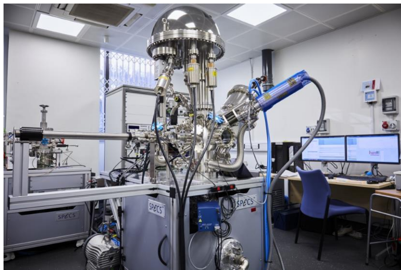
Figure 3.20 An image of the ESCA lab 250 system used in the x-ray photoelectron spectroscopy (XPS) analysis
