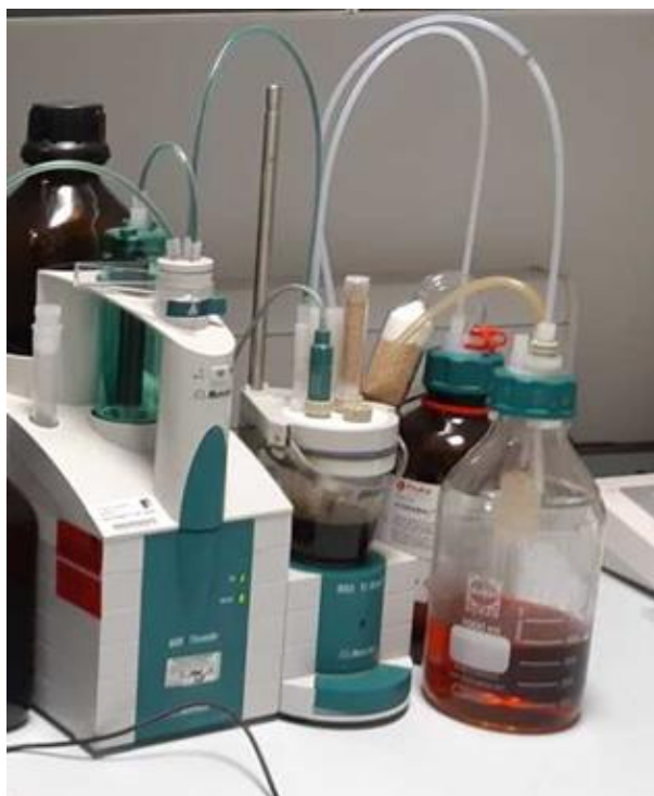
Figure 3.7 The Karl Fischer titration instrument used for bio-oil water content determination.
