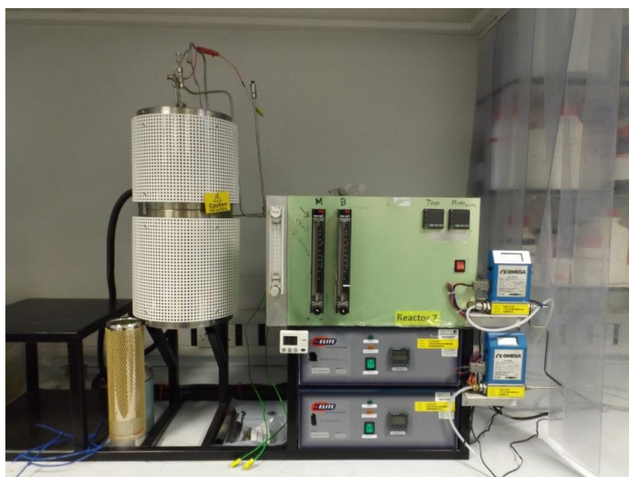
Figure 3.12 An image of the fixed bed reactor used for the slow pyrolysis process
