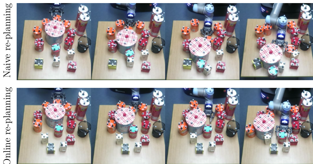
Figure 3.7: Top row: Naive re-planning (no added uncertainty) fails to grasp the target (in green). Bottom row: Online re-planning succeeds.
