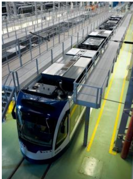
Figure 2.12: Sitrans HES installed on the roof of a train [93]
