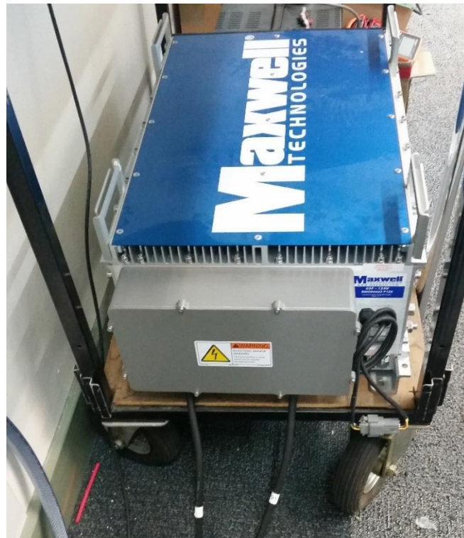
Figure 6.10: Maxwell supercapacitor module
