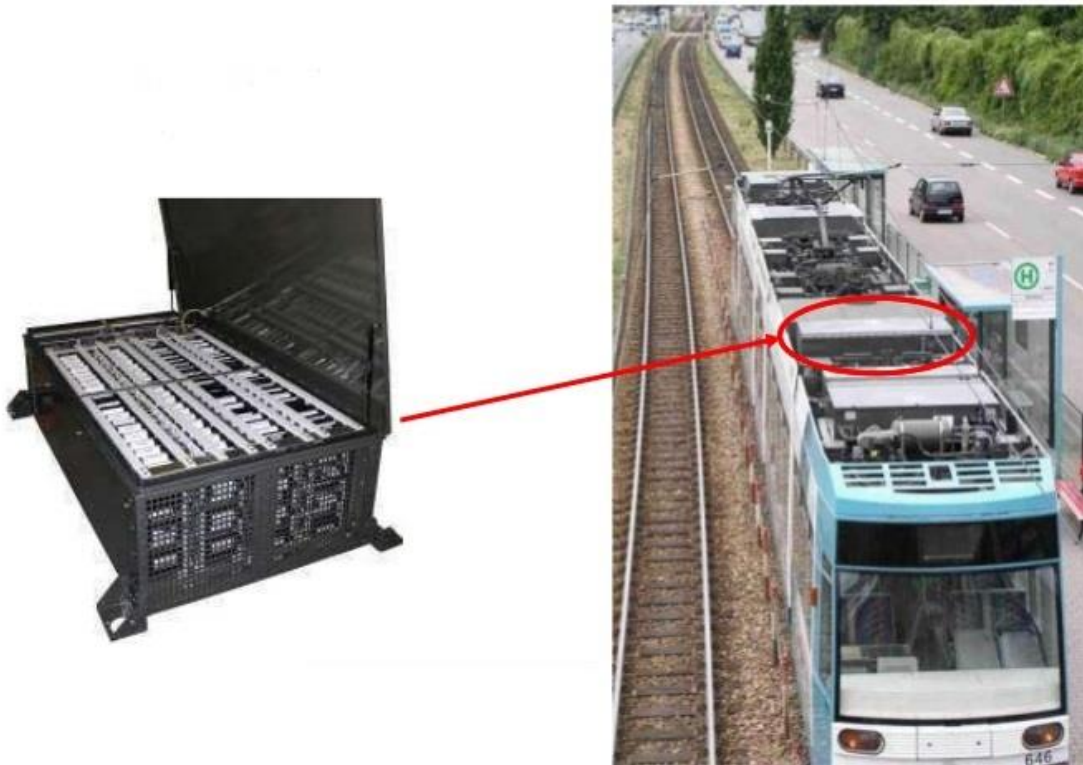
Figure 2.11: On-board supercapacitor at Mannheim Railway, Germany [9]
