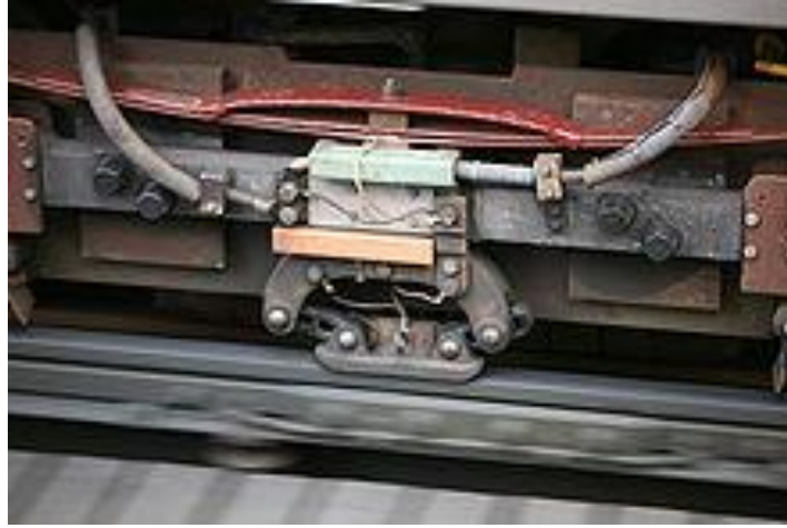
Figure 2.3: Contact shoe touching a conductor rail [44]
