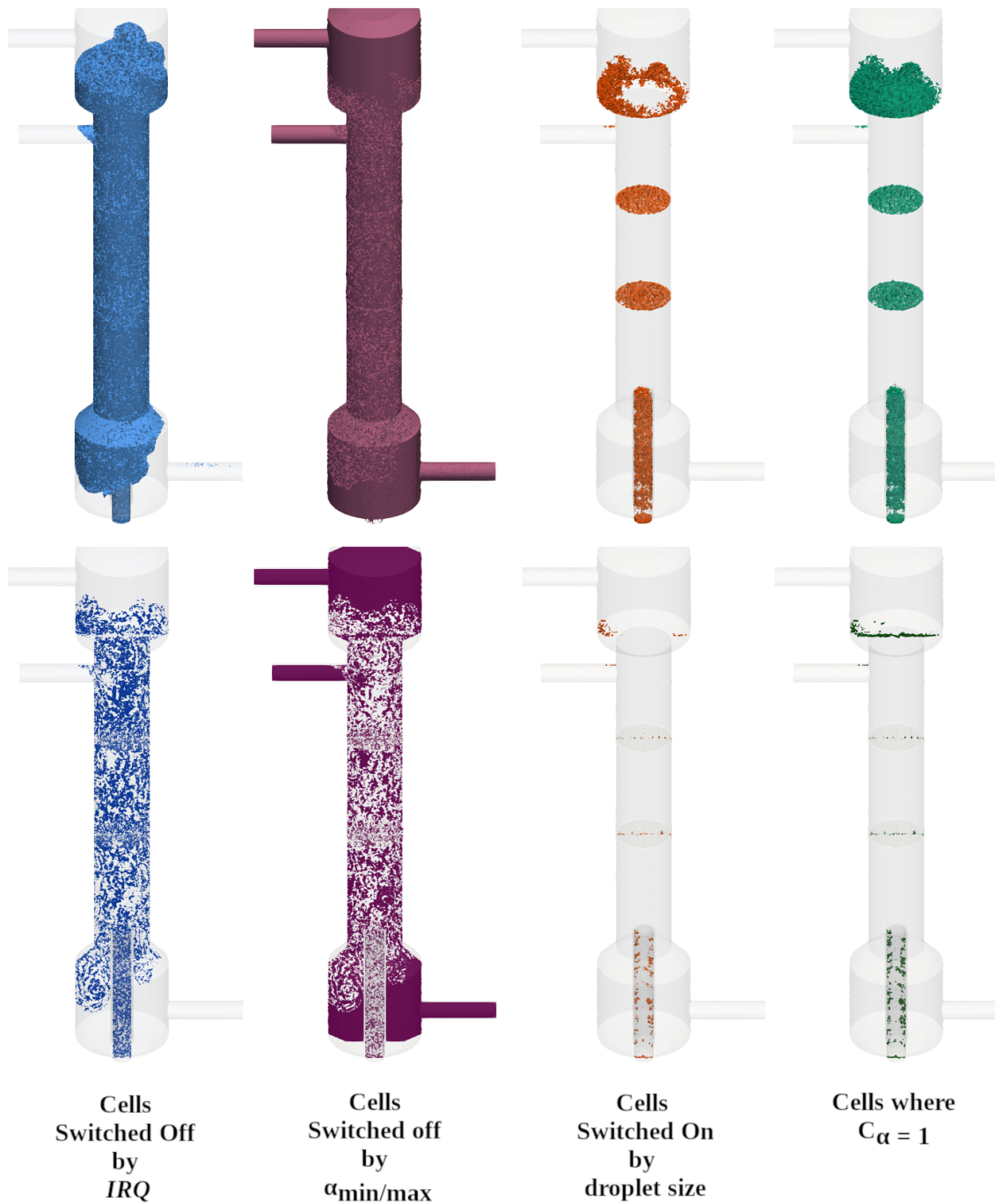
Figure 6.11: Distribution of cells switched on/off by steps in the GEMMA interfacial model switching algorithm, see Section 3.2.3.1 Fig. 3.1, at cycle time \frac{1}{2}\pi .
