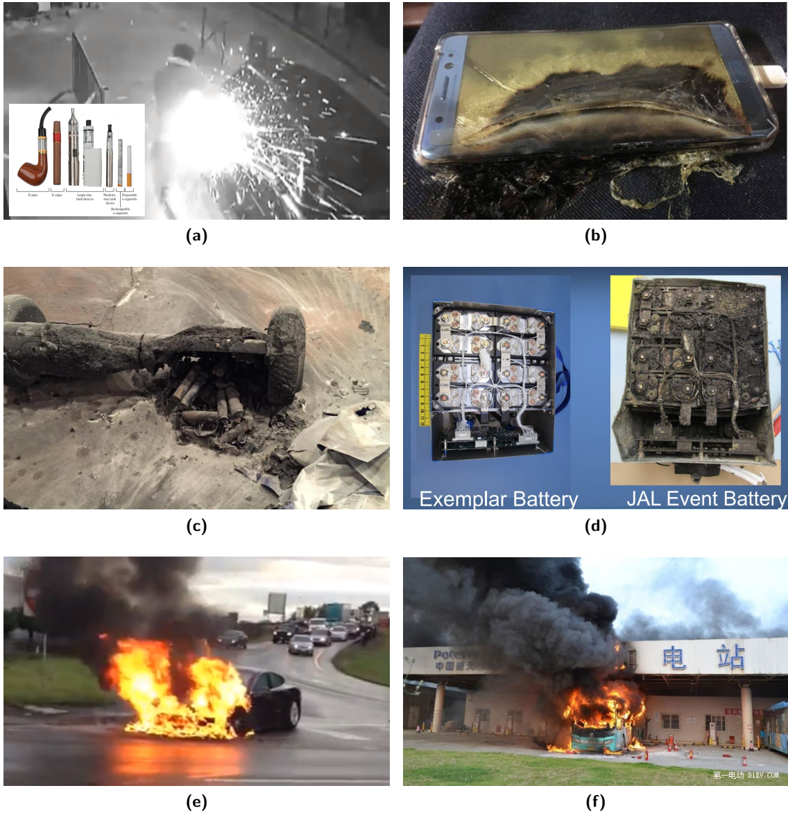
Figure 1.5: Thermal runaway incidents across various scales of battery energy capacity, (a) E-cigarette explosion in a person's pocket [44] (insert: types of e-cigarettes [45]), (b) Samsung Galaxy Note 7 smartphone post TR due to internal short due to manufacturing errors [46, 47], (c) “hoverboard” post TR while being on charge [48], (d) Boeing 787 Dreamliner auxiliary battery pre/post TR with no definitive cause known [49, 50], (e) Tesla model S on fire due to debris penetrating battery [51, 52] and (f) electric-hybrid bus on fire during charging [53, 54].
