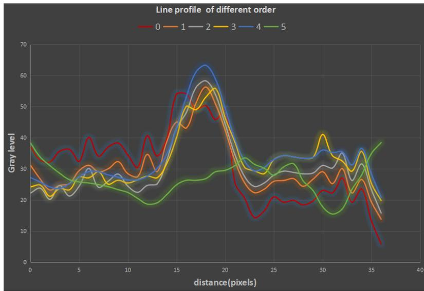
Figure 5.22: Line profiles are drawn across specific scratch characteristics under different order conditions. The horizontal axis represents the length of the line, and the vertical axis reflects the gray values at different positions.
