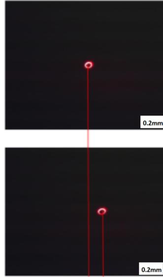
Figure 5.7: (a) is the grating to achieve horizontal deflection required by the experiment. By combining the fork gratings and the blazed gratings, and by changing the pixel period of the gratings, a grating which can realize both horizontal scanning and vortex light generation is obtained. (b) is the position of the probe corresponding to the two gratings. The red line clearly reflects the change of the position of the probe in the horizontal direction(Horizontal scanning).
