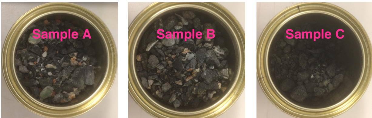
Fig. C3. Photographs of the three different unprocessed SPL samples selected for leaching trials. Sample A (left), containing a large fraction of cementitious and brick material. Sample B (middle), containing visible cementitious material. Sample C (right), appearing to be mainly graphitic material.
