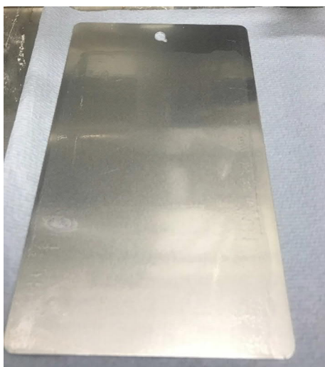
Figure 6-4 – Q-panel coated in LW17 B2 - 3 functional polymer + PT910 crosslinker after 'cure'. 1:1 ratio, stoved at 160°C for 20 minutes.
