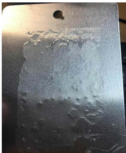
Figure 6-7 – Q-panel coating in LW17 B2 + Novolac crosslinker using 1:1 equiv. of Acid: epoxy with 0.03mol% catalyst applied with heat and no solvent, oven heated at 160°C for 20 minutes.
