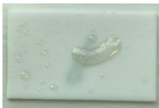
Figure 6-18 - PTFE slide containing LW17 B2 + DEN431 in a 1:1 ratio + 50% blend of EtAc/ MnAK, stoved at 160°C for 20 minutes.
