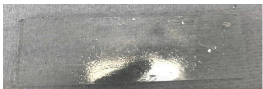
Figure 6-17 - Glass slide containing LW18 B2 + DEN431 in a 1:1 ratio + 50% blend of EtAc/ MnAK, stoved at 160°C for 20 minutes.
