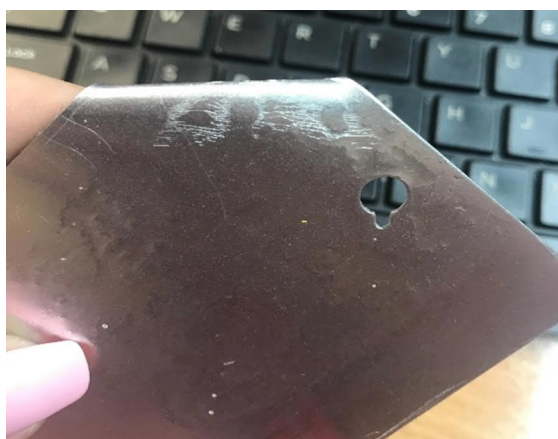
Figure 6-11 - Bend test of the Q-Panel showing LW19 (4 functional binder) + DEN431 in a 1:1 ratio +0.03mol% ETPB + 50% xylene, stoved at 160°C for 20 minutes.
