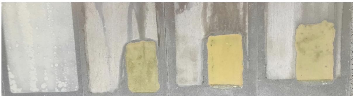
Figure 6-51 - 22 Days UV panels; Standard, LW17 (3 functional), LW18 (2 functional), LW19 (4 functional) respectively
