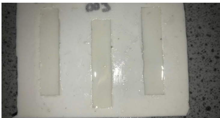
Figure 6-23 - Smaller moulds before cure showing LW18 B2 (left) and LW17 B2 (middle and right) + DEN431 in a 1:1 ratio
