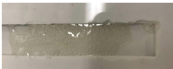
Figure 6-21 - Free film of LW17 B2 + DEN431 in a 1:1 ratio with no solvent, stoved at 160°C for 20 minutes cast in a silicone mould showing a bubbling defect
