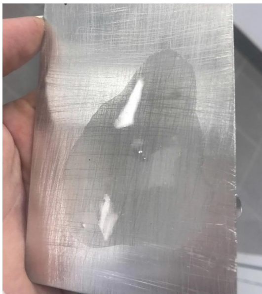
Figure 6-14 - Q-Panel showing LW19 (4 functional binder) + DEN431 in a 1:1 ratio + 50% blend of EtAc/ MnAK, stoved at 160°C for 20 minutes, after 24 hours of solvent evaporation
