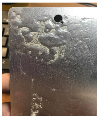
Figure 6-9- Q-Panel showing LW18 (2 functional binder) + DEN431 in a 1:1 mol ratio +0.03mol% ETPB + 50% xylene, stoved at 160°C for 20 minutes.
