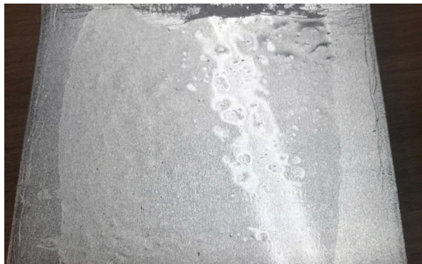
Figure 6-12 - Film of LW19 B2 (4 functional system) + DEN431 in a 1:1 ratio, with 0.03mol% ETPB in 50% THF, stoved at 160°C for 20 minutes.
