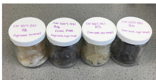
Figure 4-14 - Colour difference between polymers. From left to right high feed low heat, high feed high heat, low feed low heat, low feed high heat
