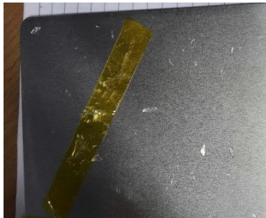
Figure 6-29 – LW17 B2 + DEN431 in a 1:1 ratio on heat proof tape placed on an aluminium Q-Panel after cure showing film cracking on removal of the tape
