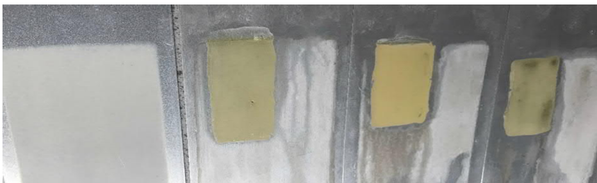
Figure 6-52 - 43 days UV panels; Standard, LW17 (3 functional), LW18 (2 functional), LW19 (4 functional) respectively
