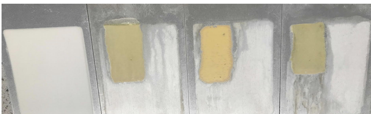
Figure 6-53 - 84 days UV panels; Standard, LW17 (3 functional), LW18 (2 functional), LW19 (4 functional) respectively
