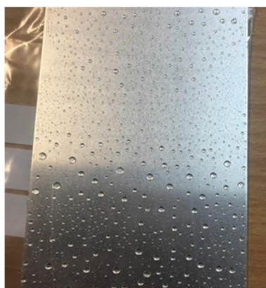
Figure 6-19 – LW17 B2 + DEN431 in a 1:1 ratio + 50% blend of EtAc/ MnAK, stoved at 160°C for 20 minutes coating on a panel containing Marbocote release agent
