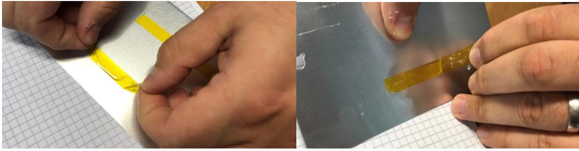
Figure 6-28 – LW17 B2 + DEN431 in a 1:1 ratio on heat proof tape placed on an aluminium Q-Panel after cure showing how brittle the coating was during tape pull off
