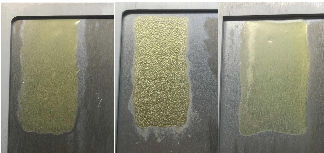
Figure 6-49 - 7 Days UV panels; LW17 (3 functional), LW18 (2 functional), LW19 (4 functional) respectively
