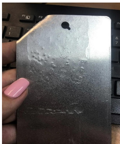
Figure 6-10 - Q-Panel showing LW19 (4 functional binder) + DEN431 in a 1:1 ratio +0.03mol% ETPB + 50% xylene, stoved at 160°C for 20 minutes.
