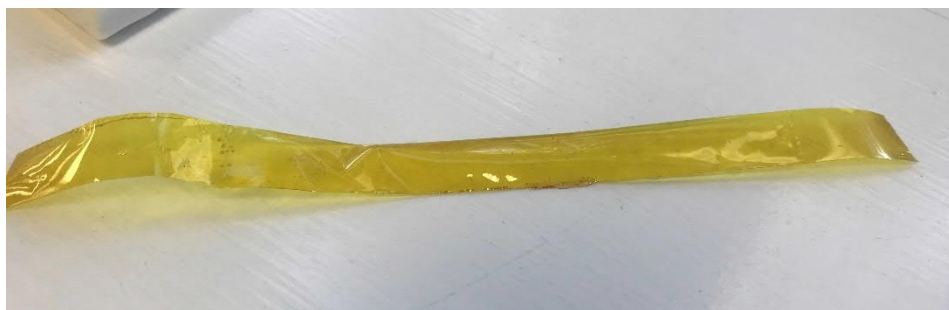
Figure 6-32 – Heat proof tape + coating removed after cure
