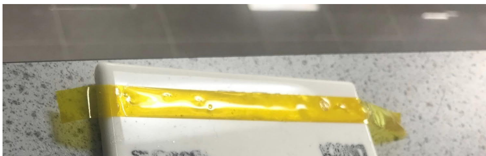
Figure 6-30 - LW17 B2 + DEN431 in a 1:1 ratio coating on heat proof tape placed on heatproof tape on a silicone mould before cure
