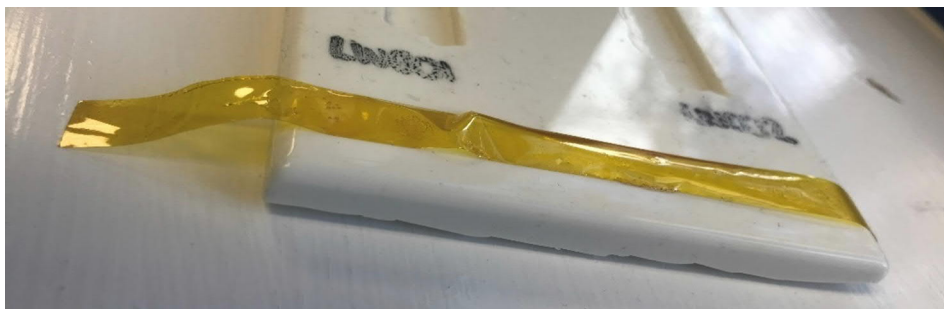
Figure 6-31 – LW17 B2 + DEN431 in a 1:1 ratio cured coating on heatproof tape
