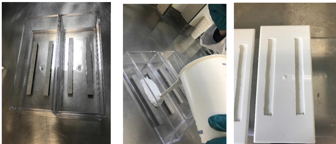
Figure 6-20 - Process of making silicone moulds to be used for making free films
