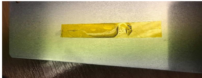
Figure 6-27 – LW17 B2 + DEN431 in a 1:1 ratio on heat proof tape placed on an aluminium Q-Panel before cure.
