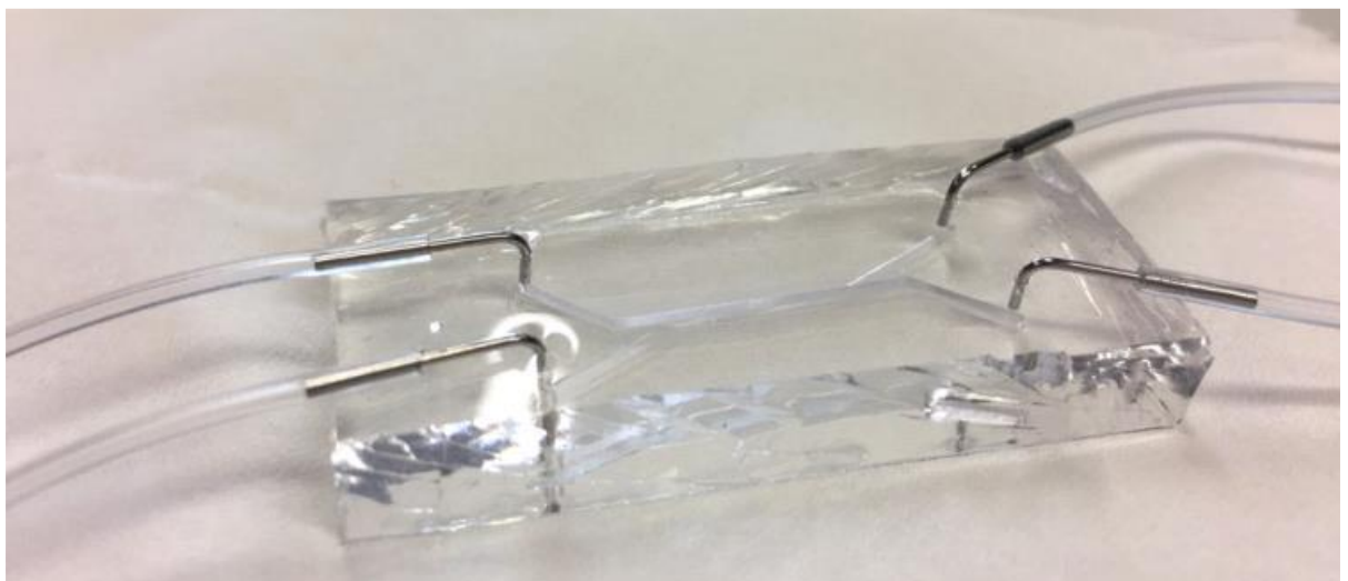
Figure 12. PDMS-based organ-on-chip 2 channel device with tubing.
