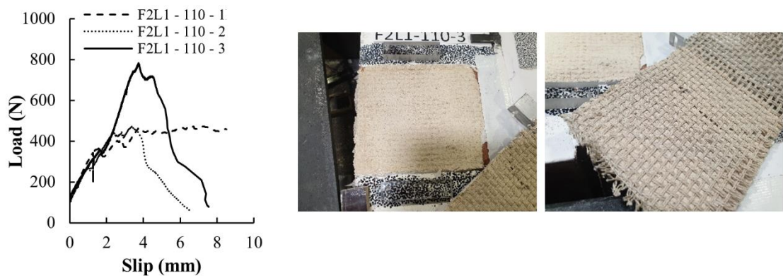
Fig. B. 3 Load-slip responses and typical failure mode of excluded F2L1-110-260 group series.
