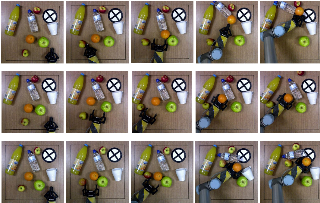
Figure 4.22: Comparing Kino-dynamic RRT (top), Greedy (middle), and VisualRHP (bottom) policies running in continuous action space in high clutter environment. The “orange” is the desired object.
