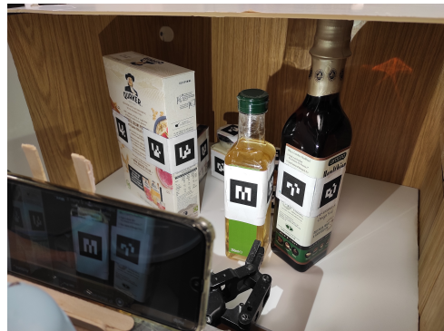
(b) Real-world: the robot is shown using a phone camera mounted on its end-effector (see Fig. 5.8 for snapshots from the camera).
