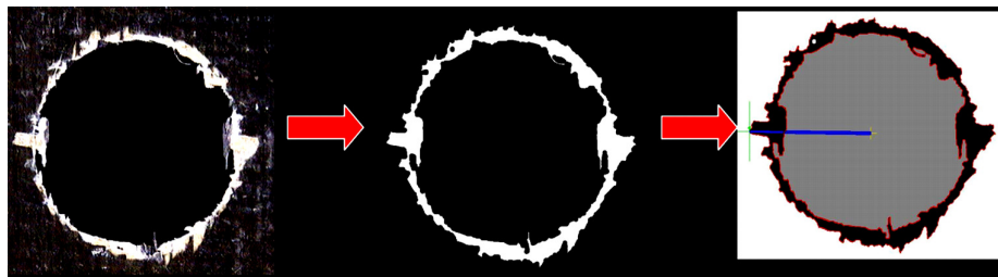
Figure 6-12: Digital Image Processing of Delamination
