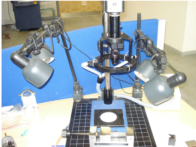
Figure 3-6: The tool microscope system
