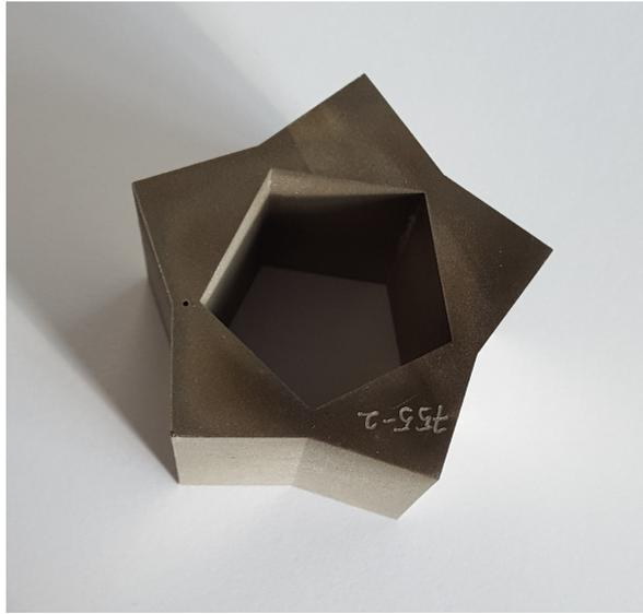
Figure 5.16: Photograph of Inconel star provide by MTC.
