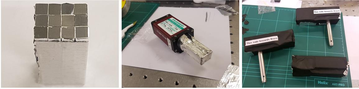
Figure 6.2: Construction process of the Mk. I module. Left: The crystals are individually wrapped in foil, then assembled into the required shape. Middle: Crystal pack is mounted to the camera, as close to the sensor as possible. Right: Light shielding is added to minimise background noise.
