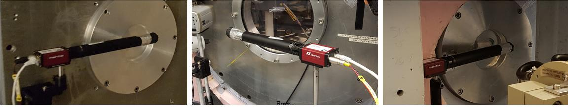
Figure 6.7: Photograph of some Mk. II scintillator modules in place outside Vulcan TAP interaction chamber.
