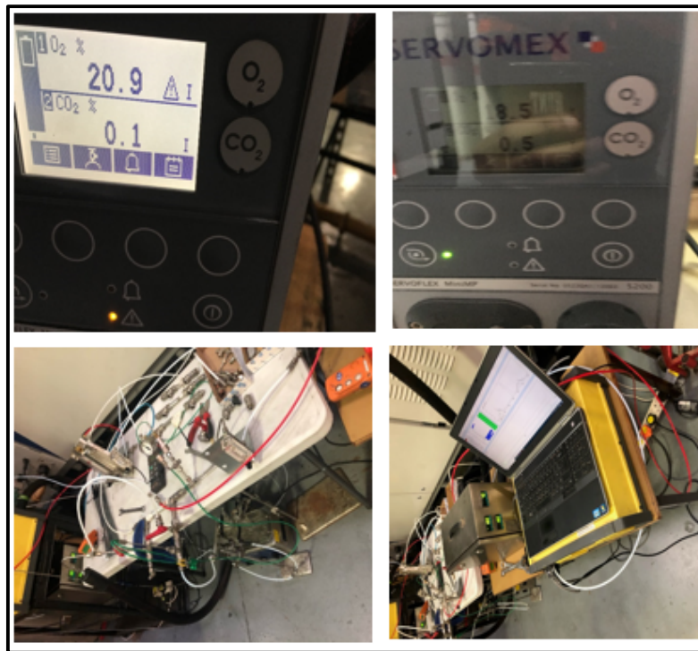
Figure 3.4: Servomex and Gaset gas analysers connected to the MGT
