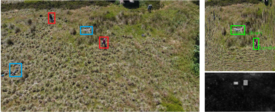
(a) Sample frame from the drone dataset, with two instances of "person lying down", in blue bounding boxes, and two instances of "person standing up", in red bounding boxes, with added artificial noise as described in Eq. 6.9
