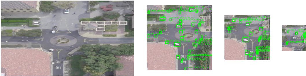
Figure 4.4: Frame from the Stanford drone dataset, at 848 \times 480 pixels, and downsampled by the described foveation approach to 416 \times 416 , 288 \times 288 and 160 \times 160 , from left to right. As the image size decreases, less objects are present in the fovea, but they are able to maintain a resolution similar to the original.
