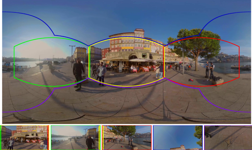
Figure 6.7: (Top) Example of an equirectangular frame, at 3840 \times 1920 pixel resolution. (Bottom, from left to right), (a) Rectilinear projection centred in [\lambda (horizontal coordinate system), \phi (vertical coordinate system)] = [0.5, 0.5] , with a resolution of 768 \times 384 pixels, and representing about 114^\circ in latitude, as illustrated by the yellow borders in the equirectangular frame (b) Projection centred at [0.2, 0.5] , green region in the equirectangular frame (c) Region centred in [0.8, 0.5] and illustrated by the red border (d) Centred in [0.5, 0.1] and bordered in blue (e) Centred in [0.5, 0.9] and bordered in purple.
