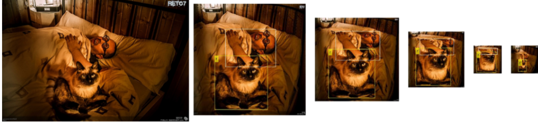
Figure 3.2: Example of typical image from the COCO dataset used for validation, from left to right, at its original resolution of 640 \times 426 pixels, at 384 \times 384 , 288 \times 288 , 192 \times 192 , and 96 \times 96 , and finally the same image normally downsampled to 96 \times 96 pixels for comparison.
