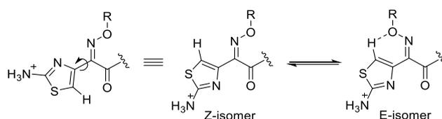
**Figure 2-8: Hydrogen bonding between the thiazole proton and oxime oxygen**
