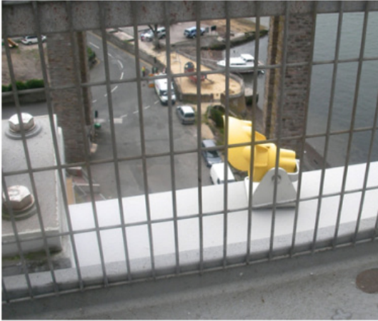
Figure 4.7: Reflector positioned on the outer beam of the cantilevers.
