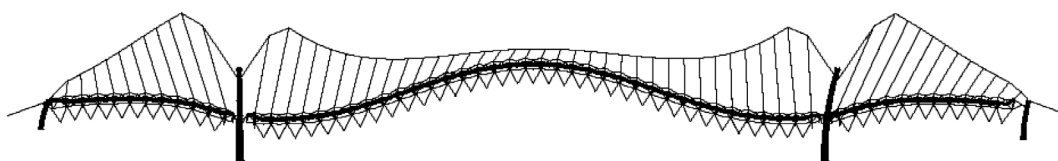
Figure 3.9: Initial configuration of the Tamar Suspension Bridge in 1961.
