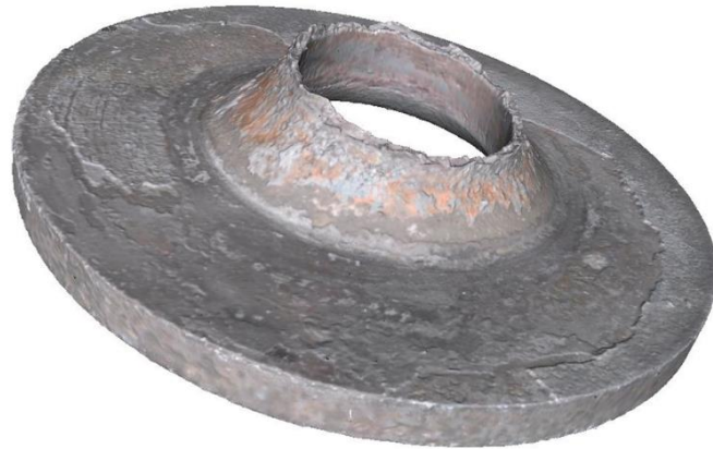
Figure 5.10: XCT scan of a fractured steel small punch test sample. The morphology of the fracture surface is indicative of a ductile failure [159].
