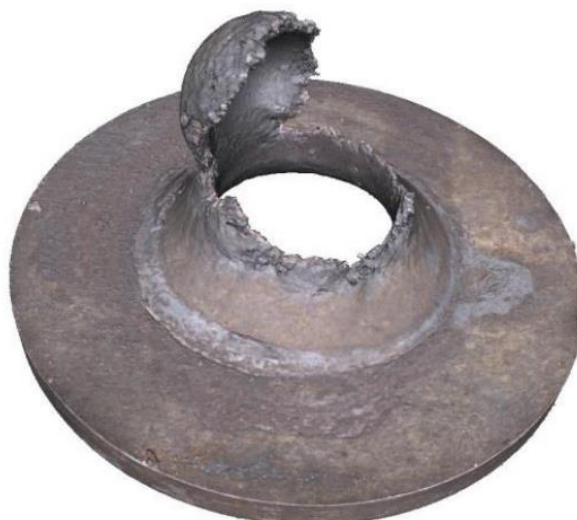
Figure 5.21: XCT scan of a fractured steel small punch test sample. Friction is essential for the formation of a cap at the top of the sample [128].
