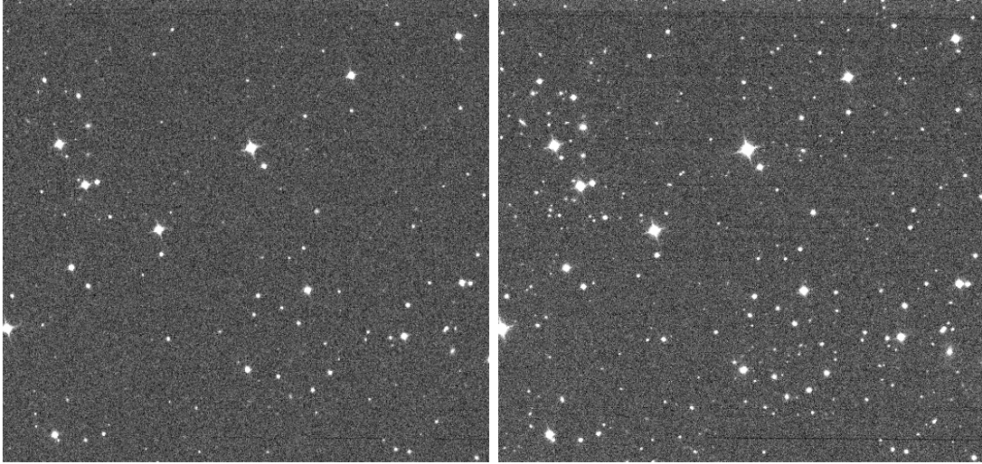
Figure 2.10: Part of a individual calibrated image (left) and the respective part of the coadd image generated from images takes in a specific range of dates (see Chapter 3). The effective exposure time of the nightly images is 180 s while the respective for the coadd images is at least 180 s.
