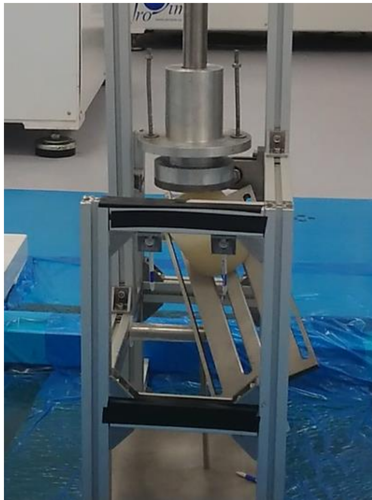
Figure 77. The collapsing platform design at the termination point of testing demonstrating the plantar flexion, inversion and internal rotation ROM of the foot plate.
