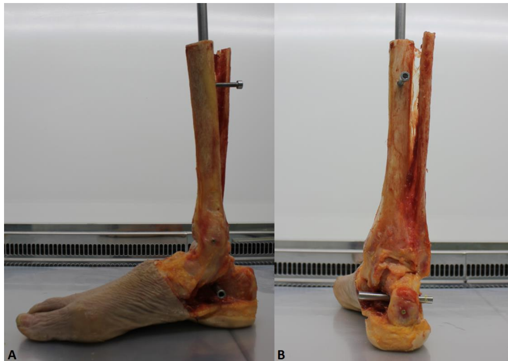
Figure 82. A) medial view and B) posterior view of a dissected sample with the intramedullary rod, calcaneal tube and medial, lateral and posterior static marker screws implanted.
