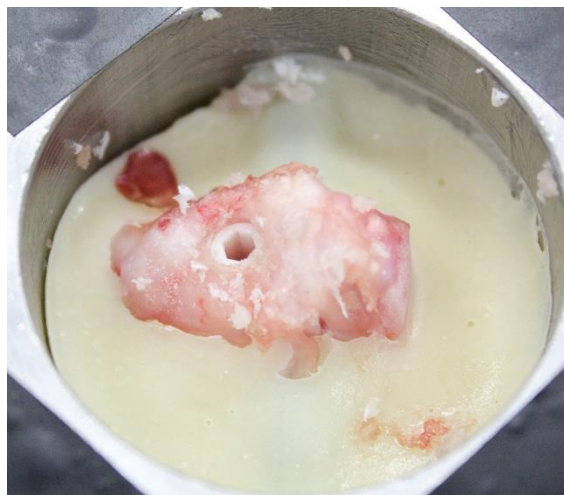
Figure 129. The porcine fibula specimen after failure of the InternalBrace suture tape.
