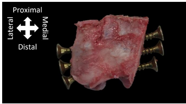
Figure 67. Porcine AiTFL sample prepared for testing following recommendations by Dr Rudert with three small (20 x 4 mm) screws into each bone piece.
