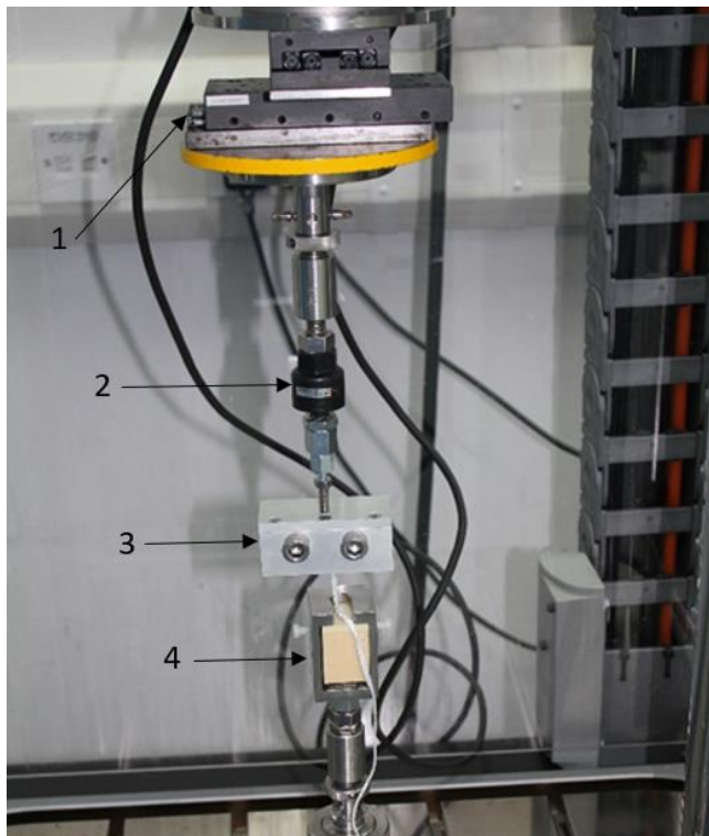
Figure 124. Testing setup showing the x-y translating platform (1), universal joint (2), interference grip (3), Infinity-Lock tape and Sawbone block within a fixed rigid grip (4).
