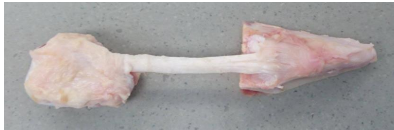
Figure 38. Bone-ligament-bone porcine patellar tendon specimen thinned to approximately 13 mm 2 .
