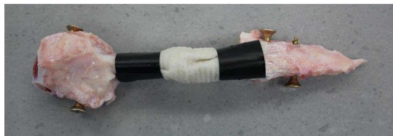
Figure 39. Bone-ligament-bone porcine patellar tendon specimen prepared for bone cementing.
