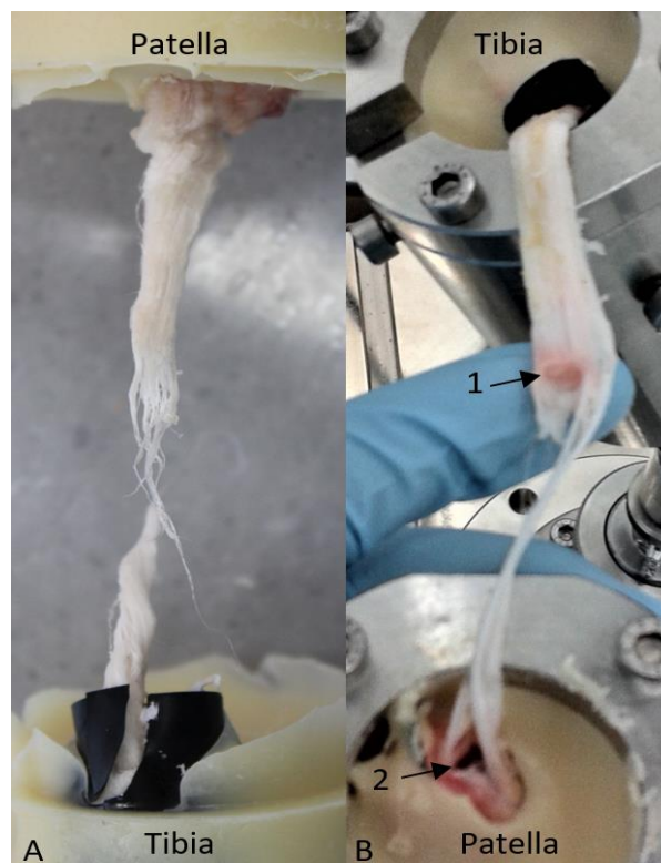
Figure 49. A) An example of a mid-substance failure for porcine patellar tendon. B) An example of an avulsion for porcine patellar tendon where a small bone fragment (1) has avulsed from the patella (2).
