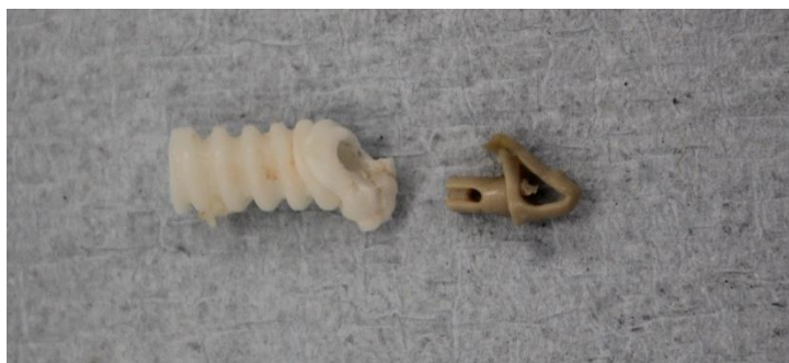
Figure 130. A failed Arthrex SwiveLock suture anchor where the eyelet has fractured and the anchor has been deformed. The suture anchor was loaded with an Arthrex InternalBrace suture tape and implanted using the tapped method described by the manufacturer.
