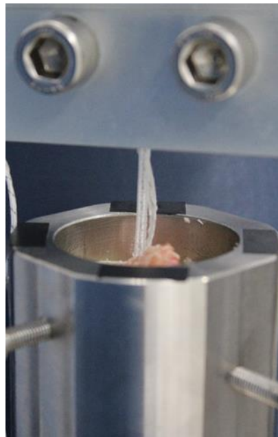
Figure 131. Arthrex SutureTape cemented into porcine fibula and both ends of the SutureTape are gripped within a mechanical grip.
