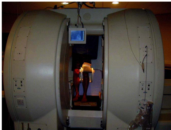
Figure 1.21 The GE 0.5 Tesla Open-access interventional MRI scanner with a 56 cm gap between magnets (Williams and Logan, 2004).
