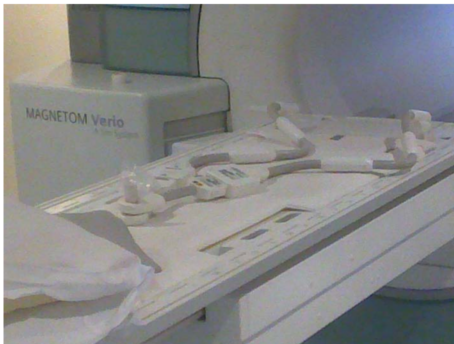
Figure 5.3 Photo shows the setting up of 3.0T MRI of a meniscus sample. The two 4-channel loop surface coils were overlapped and with their loops surrounding the sample holder to achieve best image quality.
