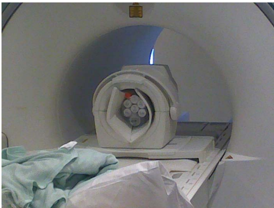
Figure 4.4 Photo of 3.0T MRI scan of multiple cartilage samples. Twelve samples were put into 6 holders and arranged in a honeycomb-like array and fixed in a 8-element knee coil, which made it possible to scan multiple samples in one time.
