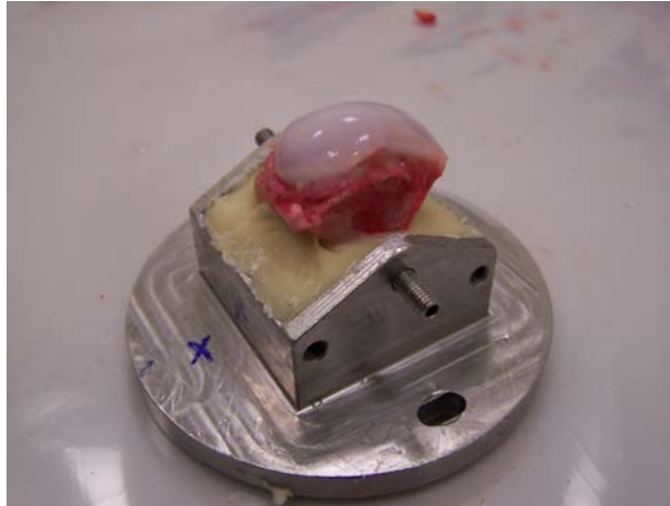
Figure 3.3 Photo of trimmed femoral condyle specimen had been set up into the jigs using screws and bone cements. The whole cartilage crown on the condyle was preserved and been kept hydrated before friction simulator testing.
