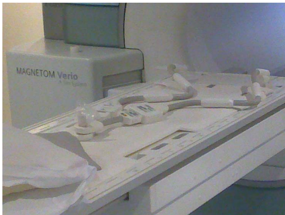
Figure 2.15 Photo of setting up of a 3.0T MRI scans of porcine meniscus sample. The two four-channel loop surface coils were overlapped and with their loops surrounding the sample holder to achieve best image quality.
