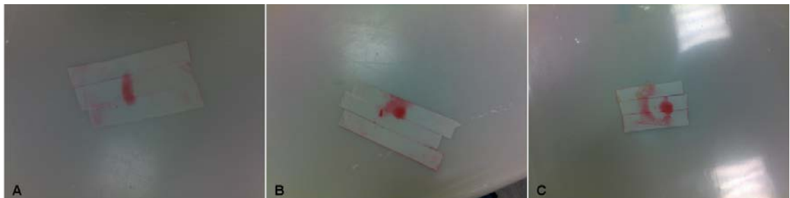
Figure 3.12 Photographs of the Fuji films after a static load of 330N was applied for 15 seconds on three models. (A) Model with intact meniscus, the contact area lay on the meniscus. (B) Model without meniscus, the density of central contact area increased remarkably. (C) Model with the inner 1/3 meniscus removed, the pink marks showed that the tibiofemoral articulation include cartilage-cartilage contact and contact between femoral cartilage with the remaining meniscus.
