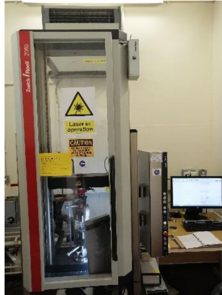
Figure 4.15 Tension machine Zwick Roell Z050
