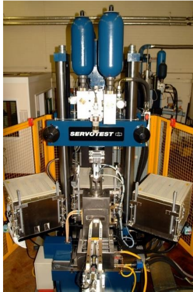
Figure 4.9 Thermomechanical compression machine for plane strain compression (PSC test)
