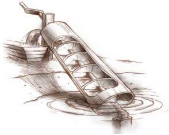
Figure 2.1 Archimedes Screw Pump (Eames, 2012)
