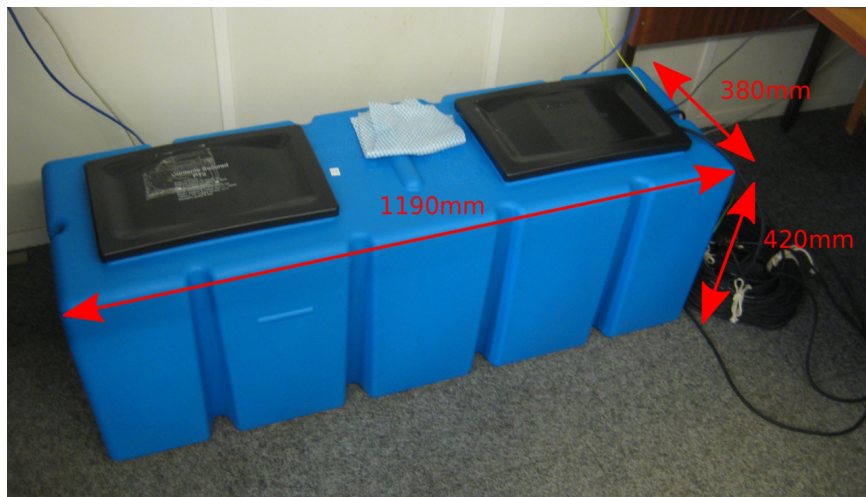
Fig. 1.12 Indoor water tank. The water tank is filled with 120 litre of water. The water tank experiments are not set up as a scaled version of the field experiment. It is used to obtain preliminary results of the cancellation scheme before the lake experiments.
