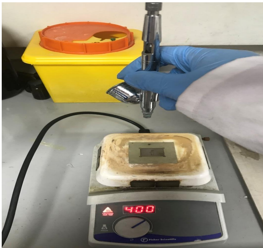
Figure 4.8: Photo of the setup used for spraying our TFT using solution precursors
