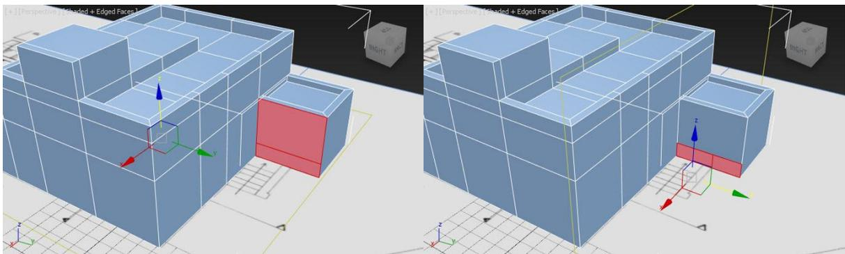
To create the entrance stairs first select the wall polygon and used the slice tool in a horizontal mode to cut the wall at an appropriate height.
