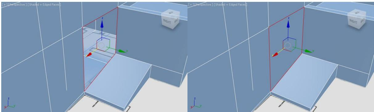
At this point the adjacent wall will overlap the stair so needs to be removed along with the inner side of the stair ramp. Before closing the open edges, it is necessary for the main wall polygon to be cut freehand along the base to match the top of the first step. The vertices at this point where the first step and the main wall intersect should be welded together allowing for the open edges to be closed using the cap tool as before.
