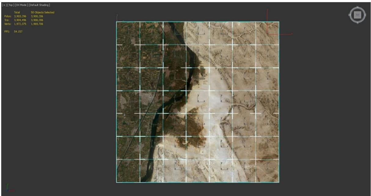
Figure 177, satellite imagery and height data exported from QGIS to 3dsmax as tiles (top view)
