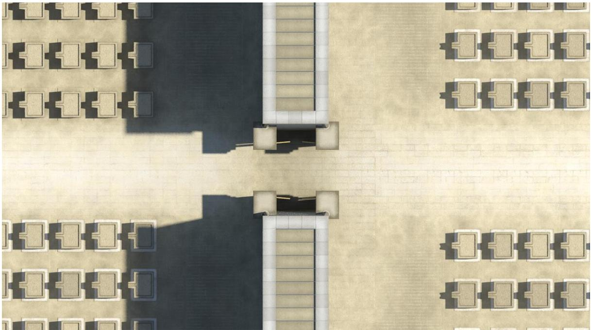
Figure 148, combined bitmap and procedural texture of the floor showing ambient occlusion used as a mask between dusty and 'walked' areas.
