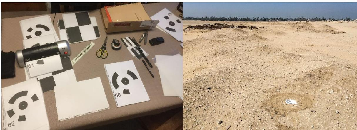
*Figure 85, photogrammetry markers being prepared (left) and in use (right)*
