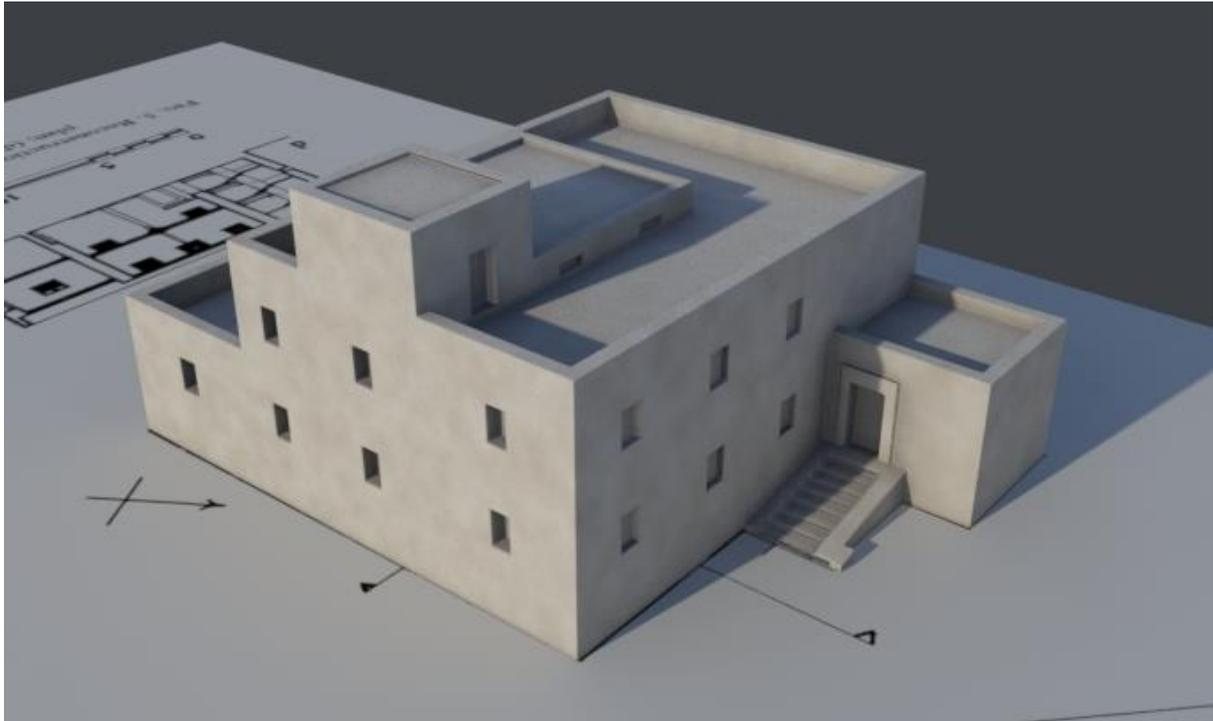
The resulting model after further work and basic textures applied. UV mapping coordinates were created using the 'UnwrapUV' modifier, selecting all the polygons, and applying box mapping followed by pack UV's using normal space to maintain a uniform size.
