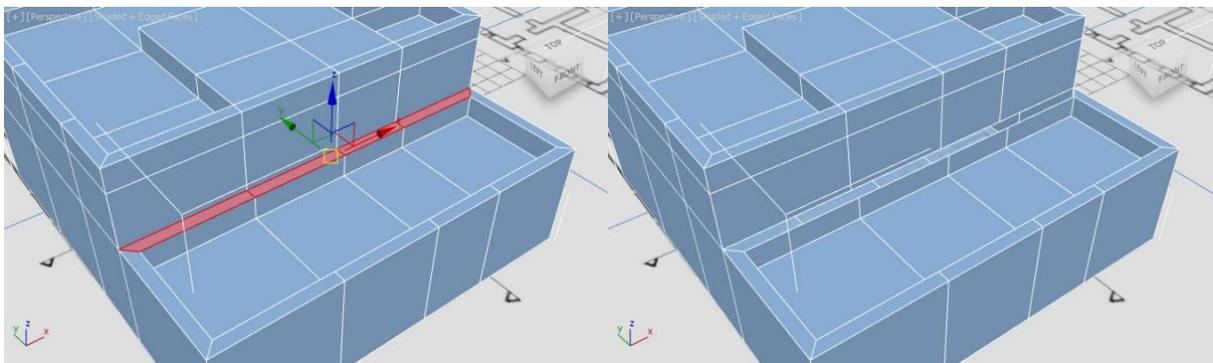
If necessary, the adjacent wall can be removed and made flush with the upper floor walls. To achieve this, select the strip of polygons and delete. In the following images the open area is closed by welding adjacent vertices using target weld. The lower rooftop vertices can then be translated to snap under the previously welded vertices creating a flush wall space.
