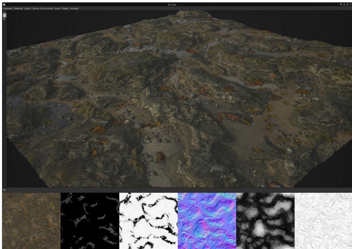
Figure 199, PBR maps (bottom left to right) used to create a physically based material (top)
