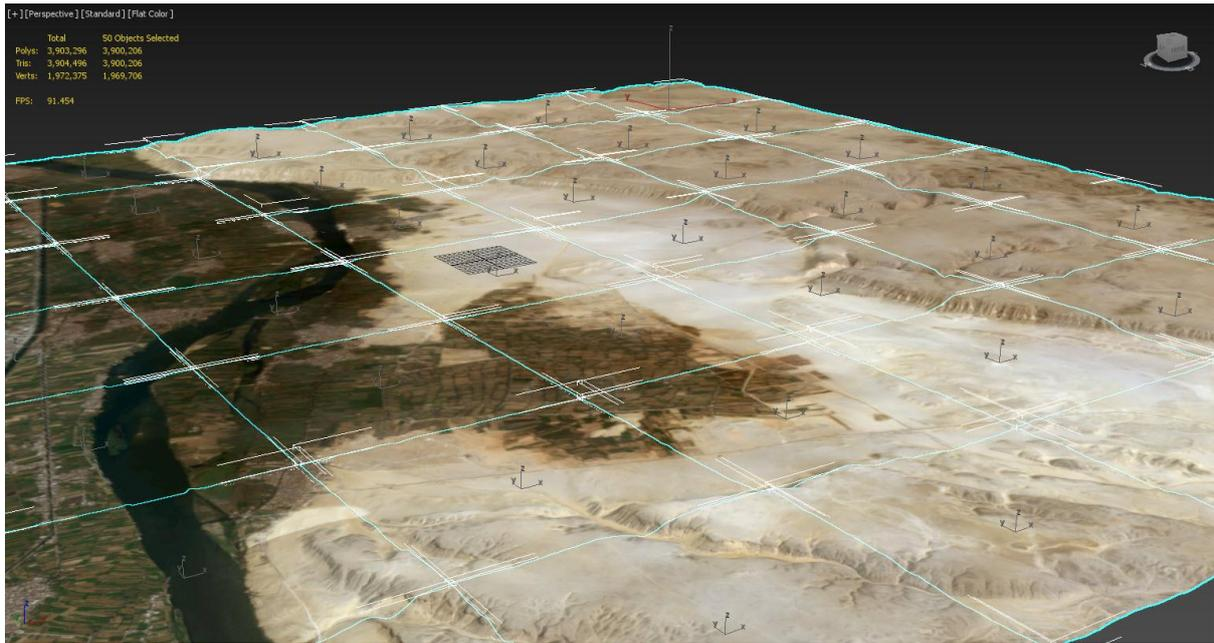
Figure 178, satellite imagery and height data exported from QGIS to 3dsmax as tiles (perspective view)
