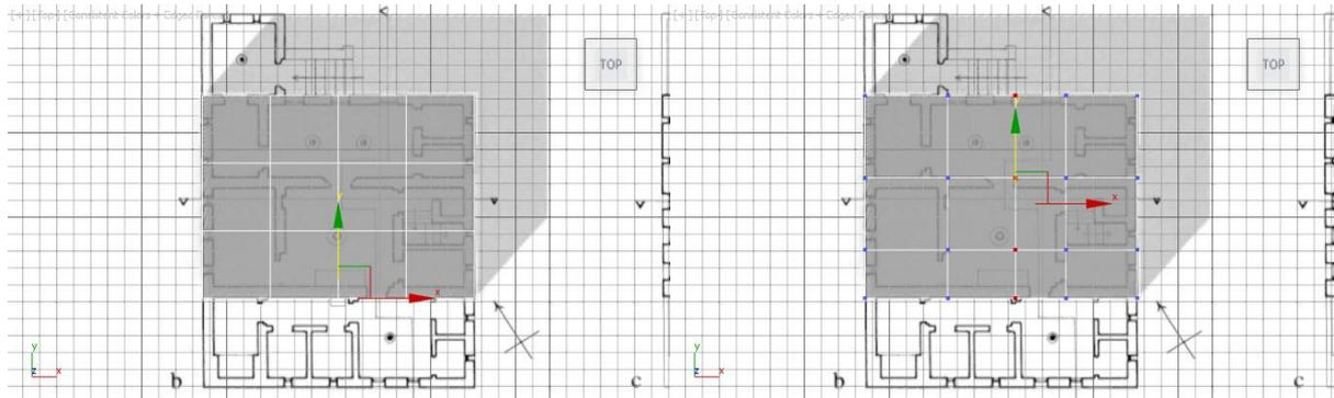
Create and position a cube with enough segments to enable extrusions based on the wall topography. Adjust the segments to follow the underlying plan by selecting loops of vertices or edges and translating them to suit. It helps at this stage to make the model transparent.
