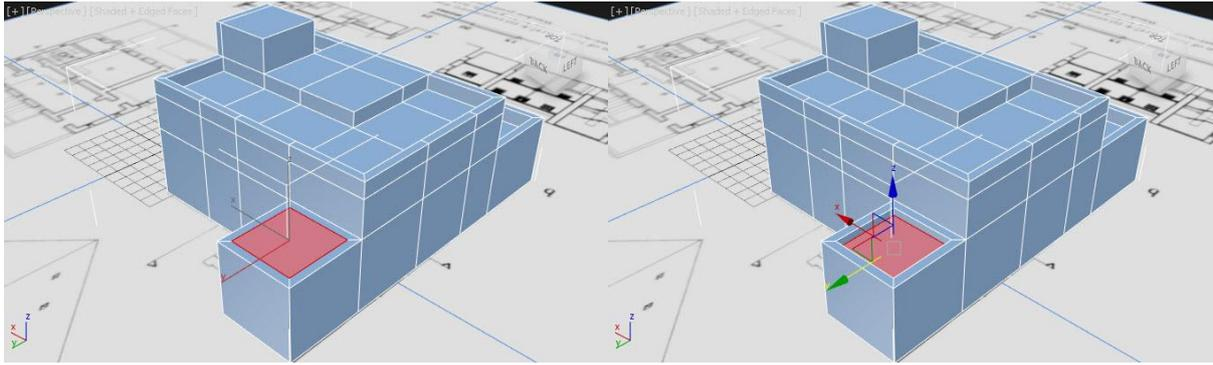
Create a short wall around the top of the porch by selecting the roof polygon, inset, and extrude downwards.
