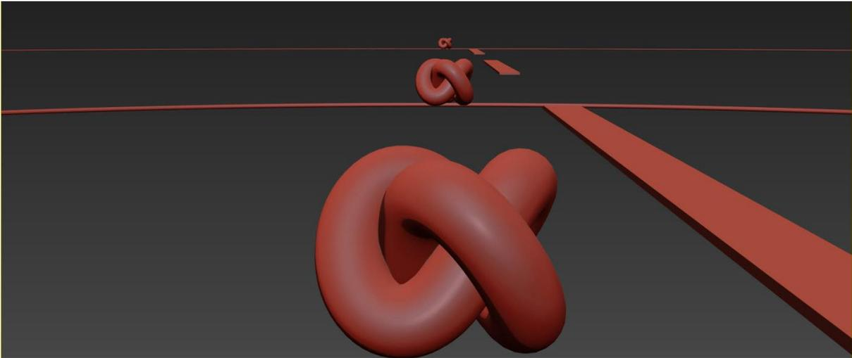
Figure 174, level of detail with distance – LoD0 (bottom) 1-unit distance LoD1 (middle) 5-unit distance LoD2 (top)
