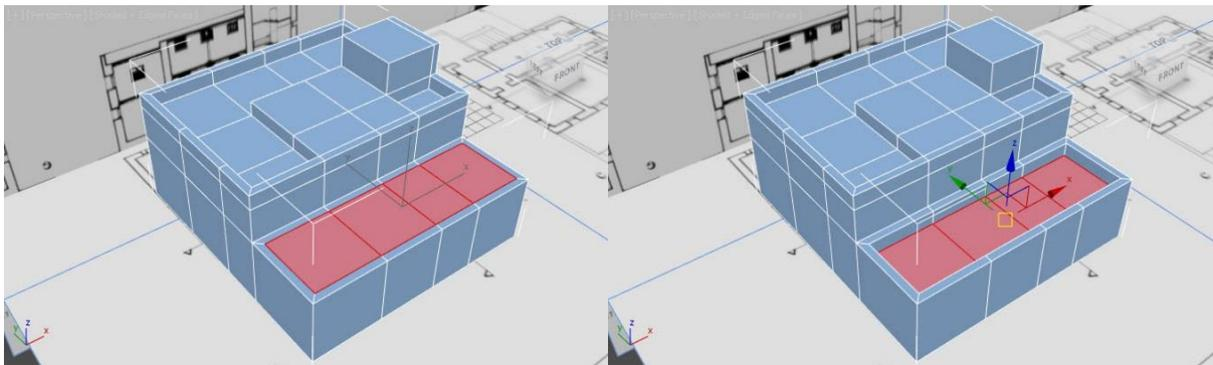
Returning to the ground floor, the roof polygons are selected and inset and extruded downwards to lower the roof and produce a short rooftop wall.
