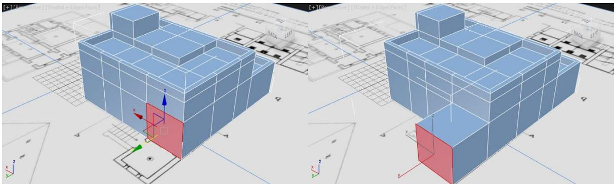
Moving around to the entrance porch of the house, select the relevant polygons and extrude as before using the plans as a guide. The stairs will be handled shortly so ignore those polygons for the moment.
