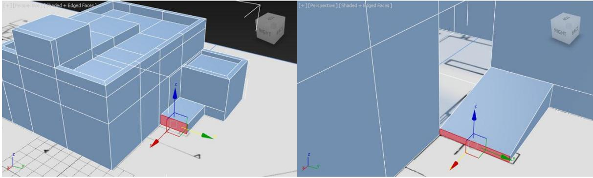
Extrude the lower polygon representing the stair and extrude out for the length of the stair using the plan as a guide. Scale the polygon down to the height of the first step by either selecting the top edge or top vertices and translating downwards.
