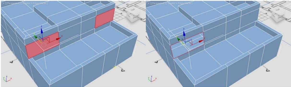
The previous action will have created open edges where the lower roof wall rim meets the upper floor. This can cause problems later when texturing and rendering the model so to fix this select the upper polygon and delete it. Then select the open edges and use the cap tool to rebuild the polygon without any open edges.
