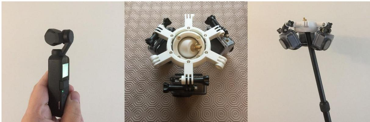
*Figure 86, photogrammetry equipment. DJI Osmo Pocket (left), custom action camera rig (middle & right)*
