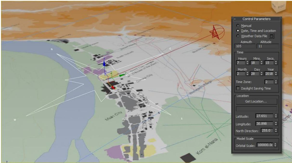
Figure 159, view of the sunlight system in 3dsmax using a proxy map for initial setup
