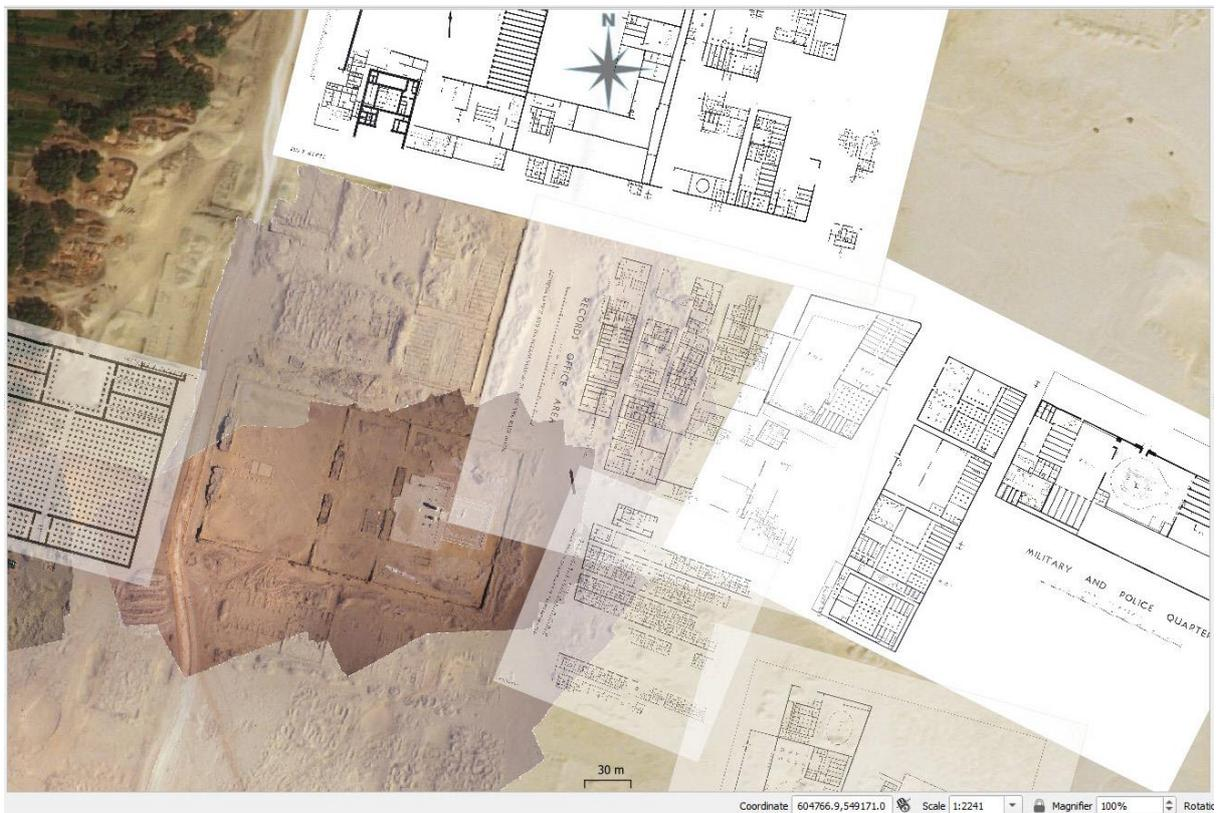
Figure 23, a selection of orthographic photography and georeferenced plans at different transparencies to show layering.
