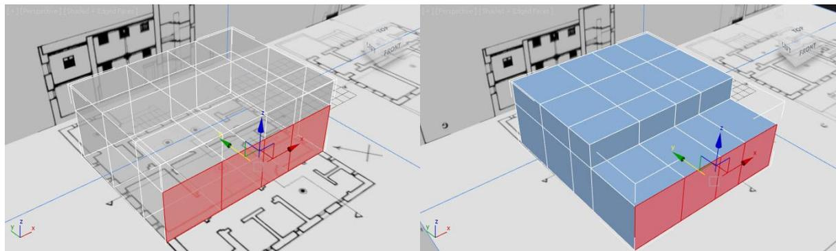
In this example the lower segments/polygons represent the ground floor which are selected and extruded to match the plans.
