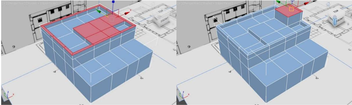
The selected polygons are extruded to a height representing the upper walls and, in this instance, polygons representing the stairwell are selected and extruded to the appropriate height.
