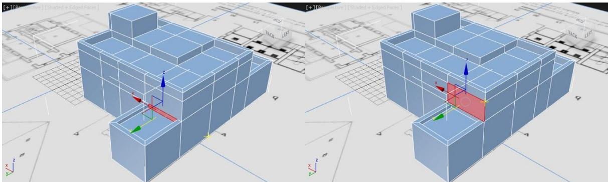
The adjacent wall can be made flush in the same manner as earlier by removing the upper polygons, adjusting the vertices, selecting the open edges, and using cap to rebuild the wall polygon.
