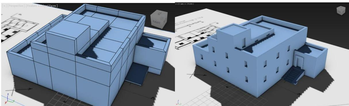
You will now have a solid model in the shape of the Amarna house which can be further modified using combinations of inset and extrusion (for doors and windows) along with slice and chamfer (in the case of the stairs) resulting in the model shown above right.
