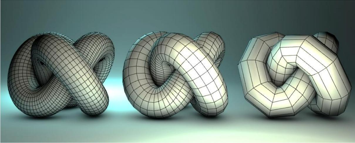
Figure 173, level of detail example – LoD0 11,136 polygons (left) LoD1 2880 polygons (middle) LoD2 840 polygons (right)
