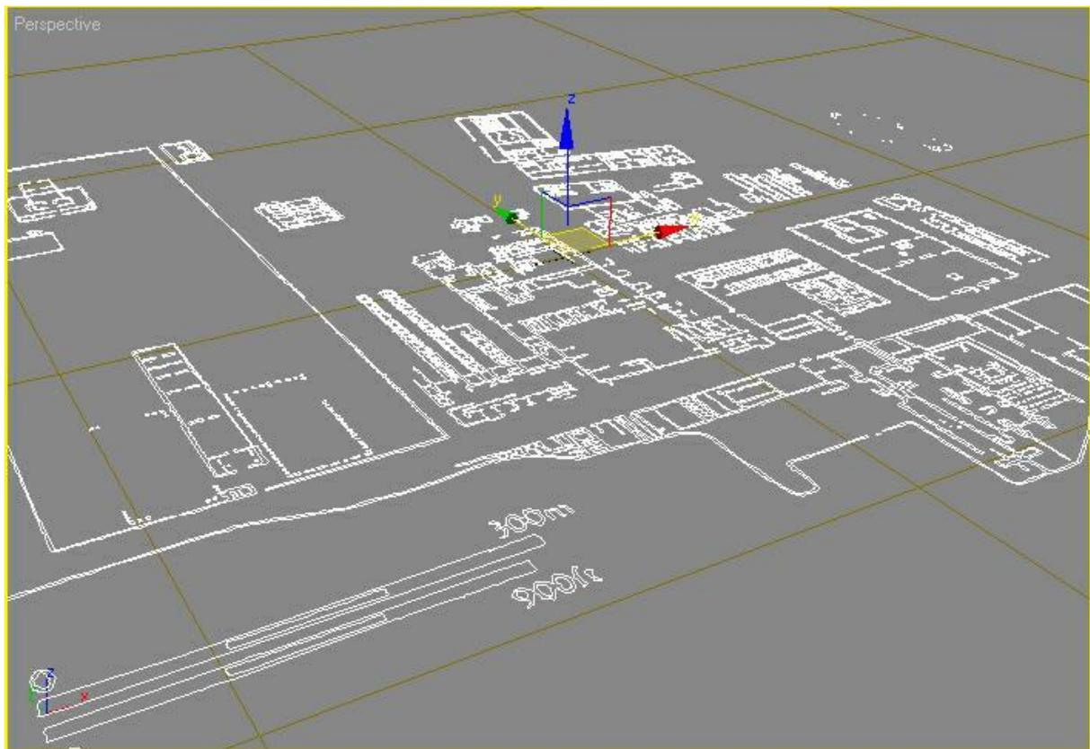
*Figure 114, Central City plans imported into 3dsmax as construction guide*
