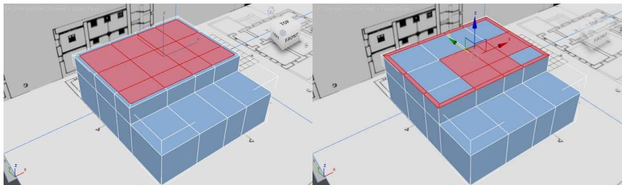
The roof segments/polygons are selected and inset to provide an outer frame from which the upper boundary wall will be extruded later. This frame is selected along with the polygons relating to the central room.
