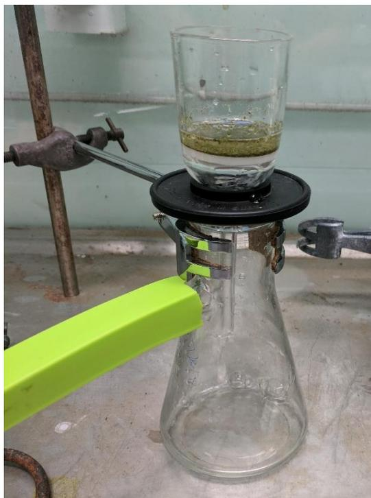
**Fig. 1S.** Washing on a glass filter from the excess of chloride anions
