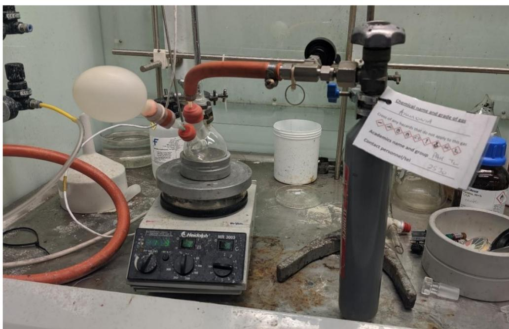
Figure 94. The set-up for ammonia adsorption on the catalysts surface
