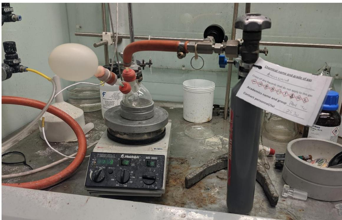
FigureS5. The set-up for ammonia adsorption on the catalysts surface
