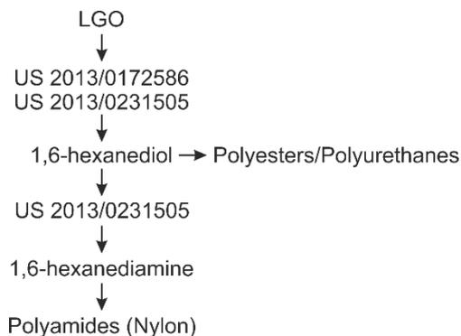
Figure 15. Application of the levoglucosenone as an intermediate for polymers
