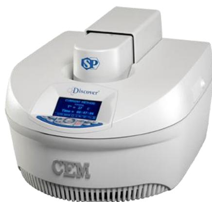
**Fig. 4S.** The microwave reactor – CEM Discover
