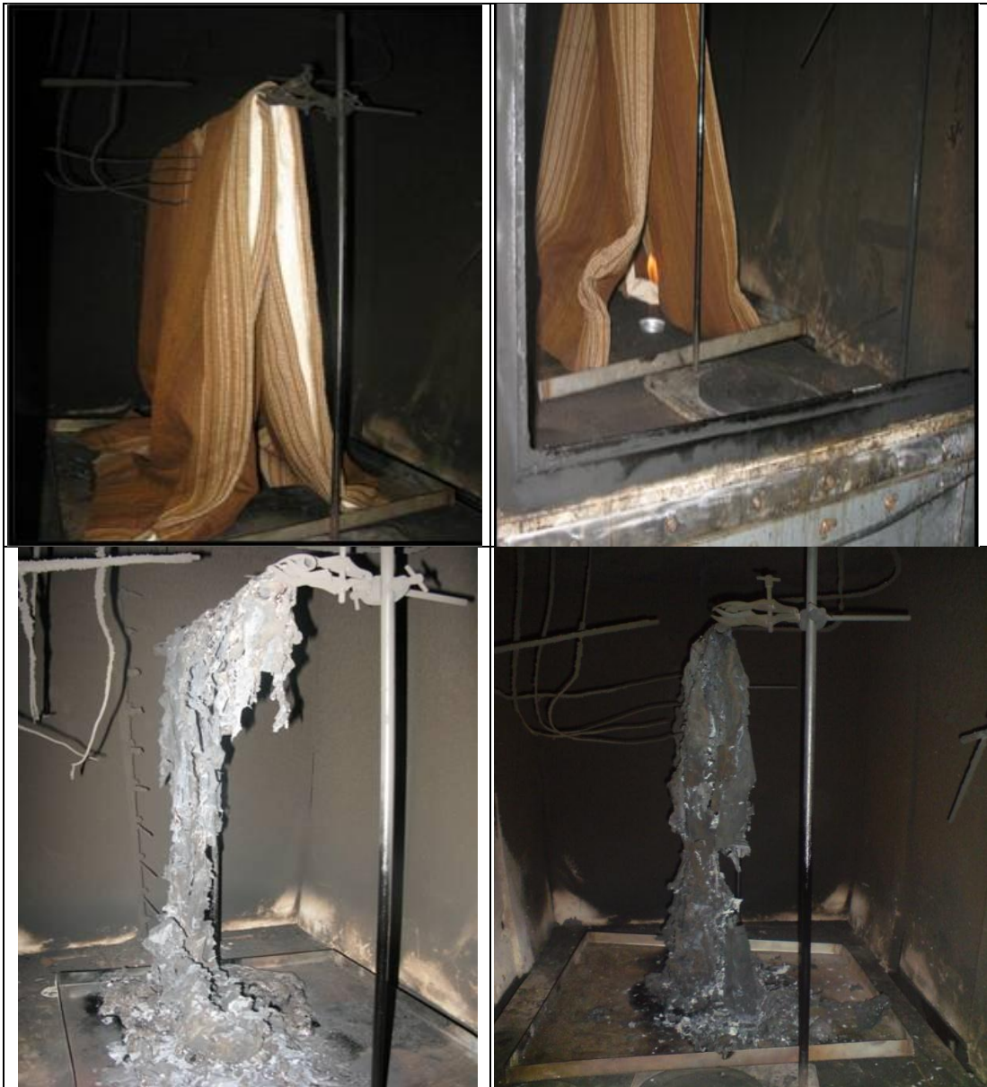
Figure 7-1: Pictures of the curtain set up, ignition, debris after the four fires.
