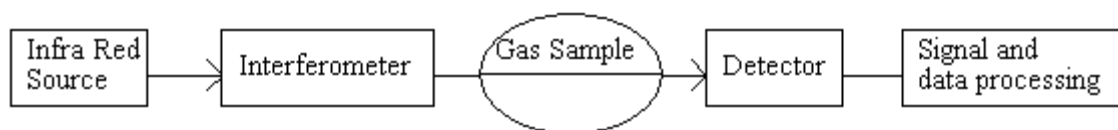
Figure 3-10: A sketch of the basic FTIR components.
