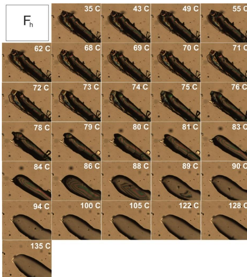
Appendix Figure C.9: Hot-stage micrographs of a single F_h crystal heated from 35 to 135 °C at a rate of 5 °C \text{min}^{-1} . Originally in colour.
