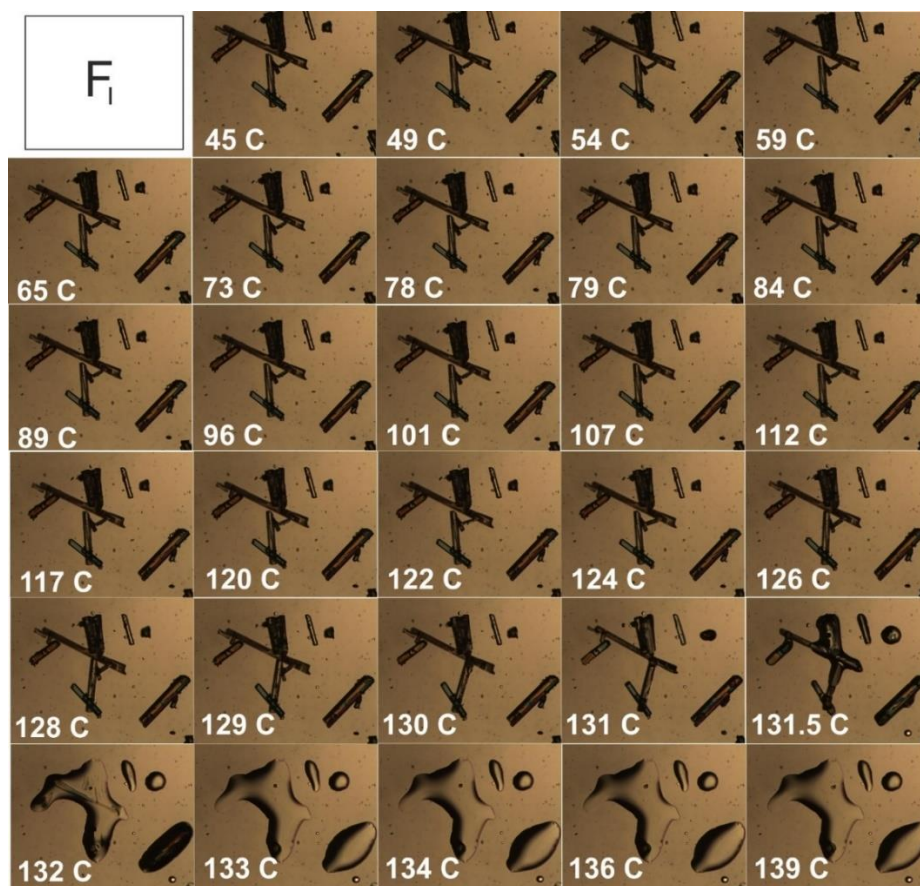
Appendix Figure C.7: Hot-stage micrographs of a single F_1 crystal heated from 45 to 139 °C at a rate of 5 °C min -1 . Originally in colour.
