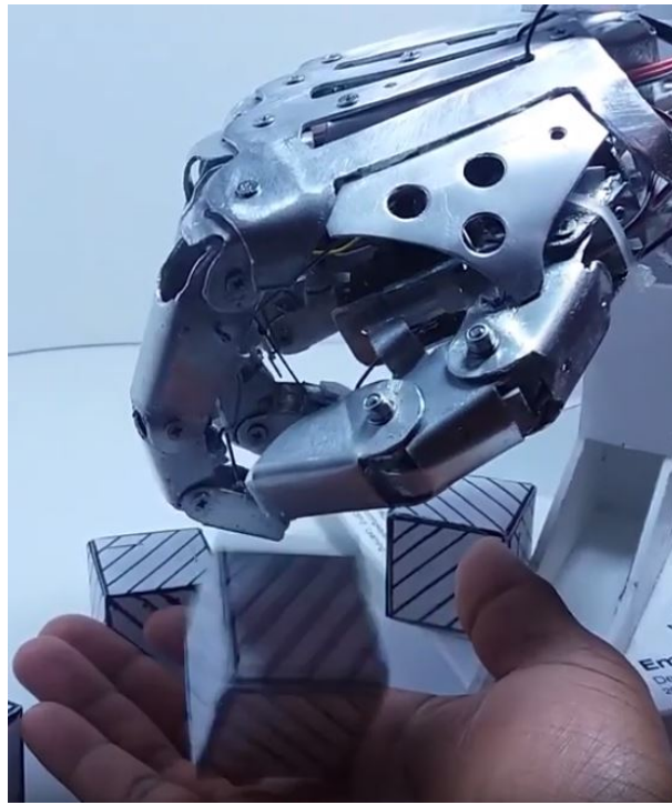
Figure 4.4: Assistive robotic prosthetic hand stacking blocks.
