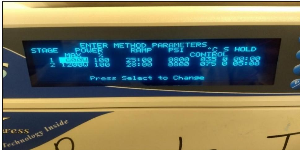
Figure 3.19 Operational conditions of the MARS Xpress and an example of the microwave irradiation programme used to pre-treat digestate.
