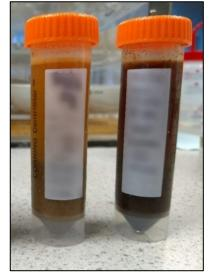
Figure 8.3 Food Waste samples from a same microwave run treated at 175°C 1.9°C/min, showing different colours, possibly due to differences in distribution of the electric field. Picture: Mariana Turnell (2018).
