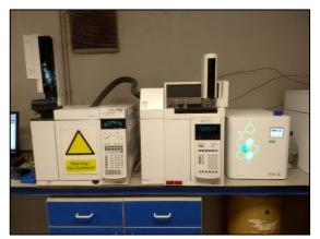
Figure 3.8 Gas chromatograph (Agilent 7890A) at the IPHEE laboratory, Civil Engineering Leeds University.
