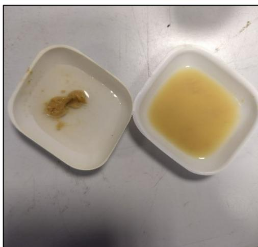
Figure 3.14 Solids dilution (2 g) prior to microwave irradiation.
