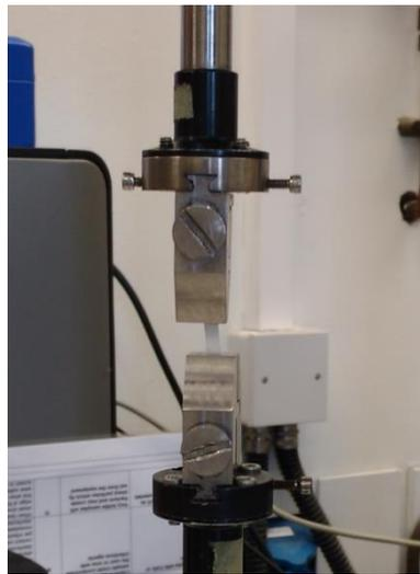
**Figure 2.2** Strip of a PLGA scaffold being tested in the tensiometer.
