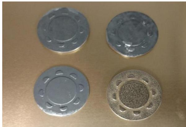
**Figure 4.7** Different thickness of metal collectors. 1 mm (down left), 1.5 mm (upper left), 2 mm (upper right), and 3 mm (down right).
