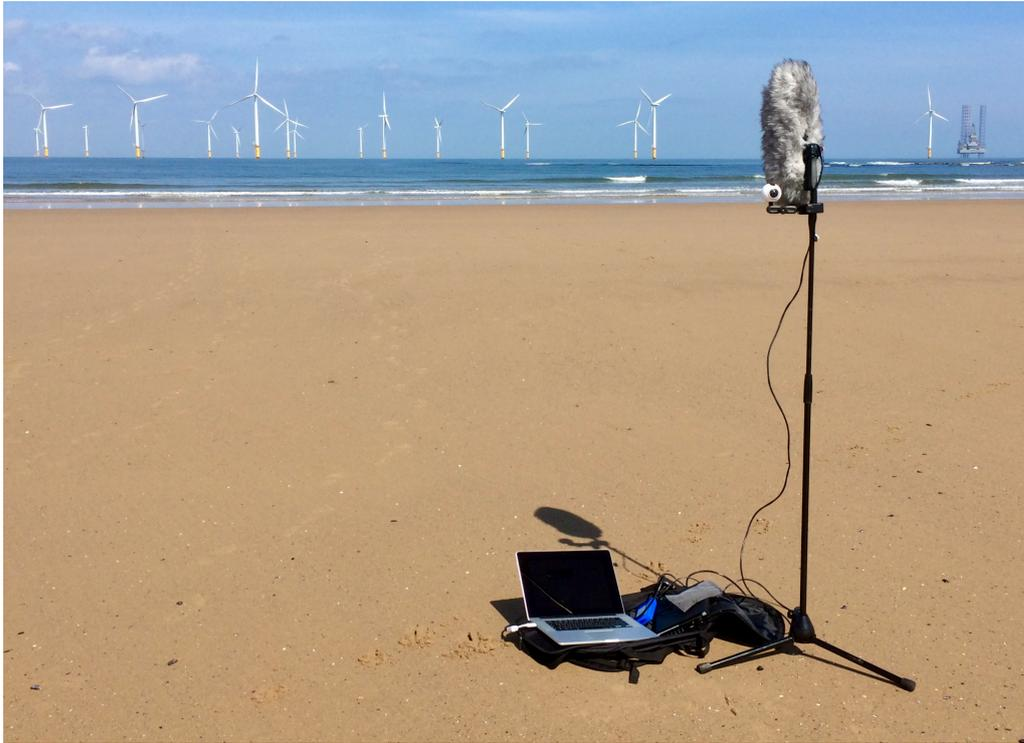
Figure 5.2: The EigenScape recording setup at Redcar Beach, North Yorkshire (recording of Beach-04).
