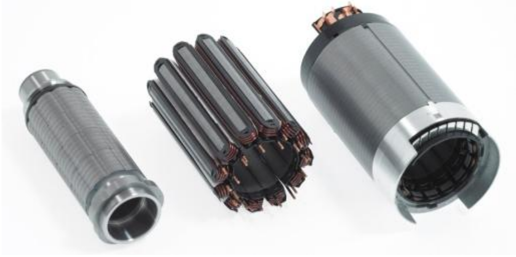
(c) Prototype rotor and stator, together with wound stator teeth stack before insert into stator yoke
