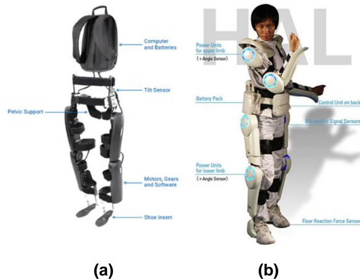
Figure 2.10: (a) Rewalk Exoskeleton [3] (b) HAL by Cyberdyne Inc. [28]
