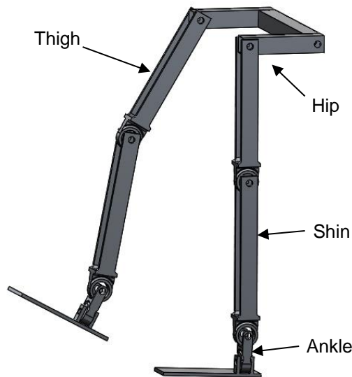
Figure 4.3: Model of the Lower Limb Exoskeleton representing the hip, knee and ankle joint.
