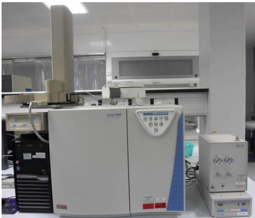
Figure 3.11. Thermo Scientific Flash EA2000 elemental analyser.
