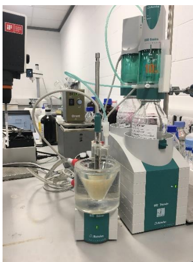
Figure 2.7 Metrohm pH stat titration system consisting of two dosing units, pH sensor with temperature monitoring and a 60 mL jacketed reaction vessel connected to a heated water bath circulator sat on the stirrer unit.
