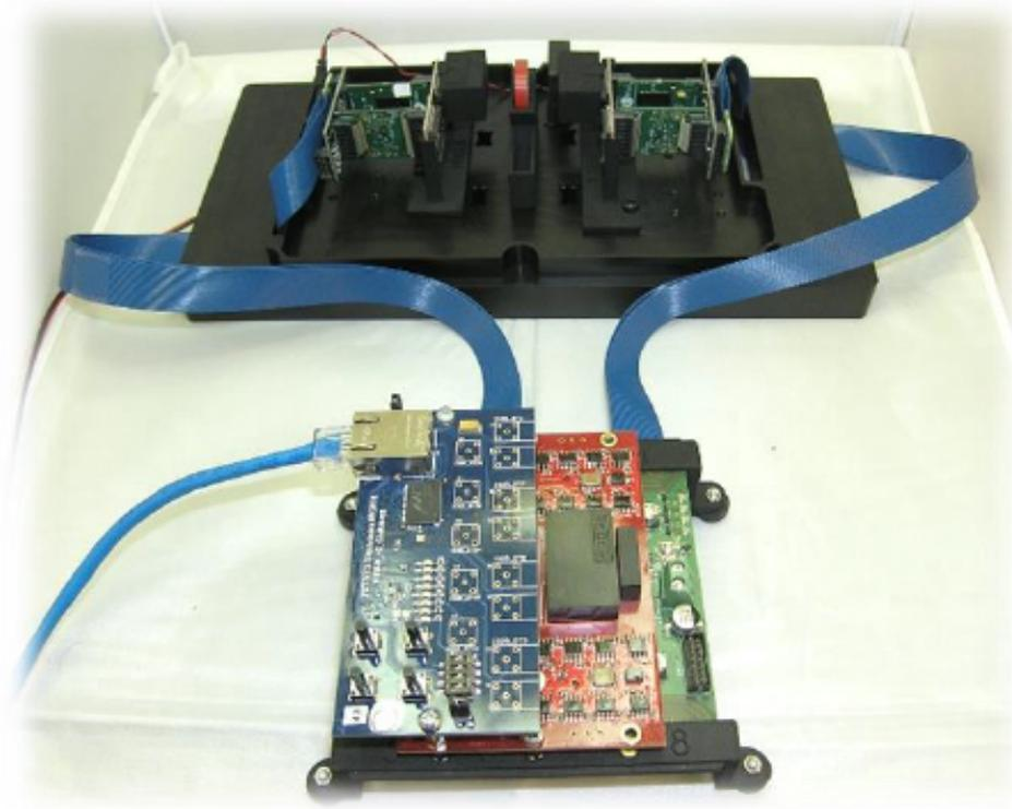
Figure. 3.12 The ASICs setup connected with the SiPMs of two small LYSO detectors for coincidence measurements.
