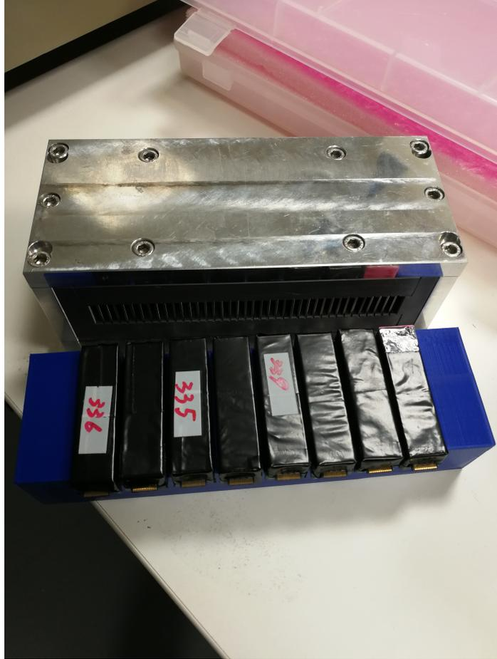
Figure. 3.4 A photography of the multi-slit collimator with eight LYSO detector arrays arranged behind its slits, leaving one every five slits without being seen by the detectors..
