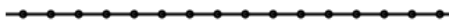
Figure 3.1: A Toda lattice made from sites with equal mass m , equal separation L , connected by Toda potential.
