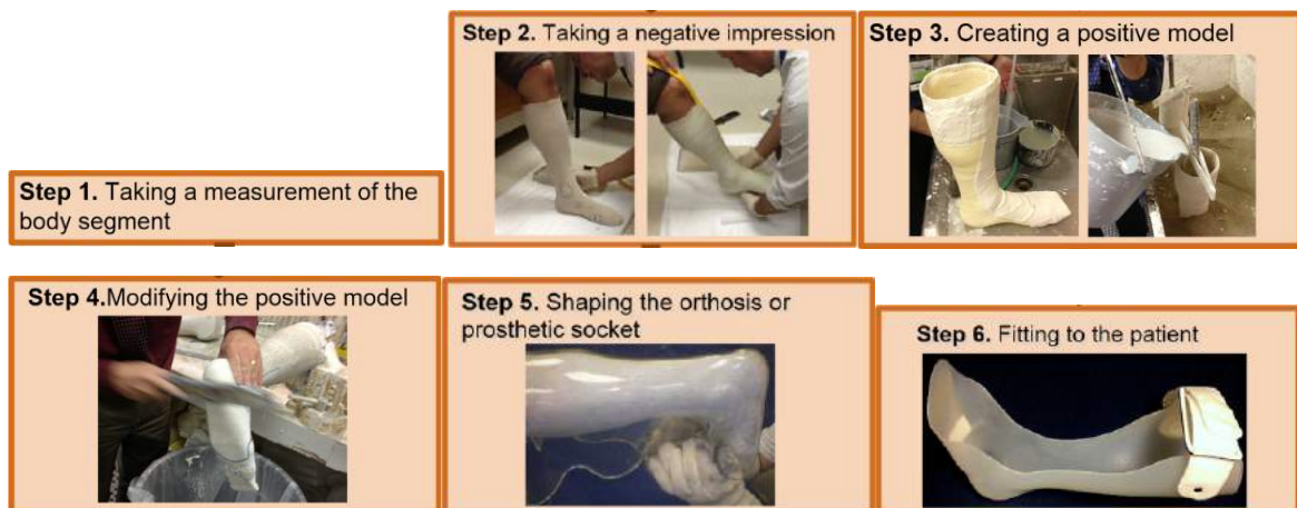
Figure 2.3 - Manual process for producing an ankle-foot orthosis [62]
