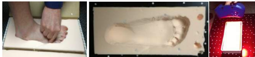
Figure 2.5 - Foam impression box and 3D scanning [62]
