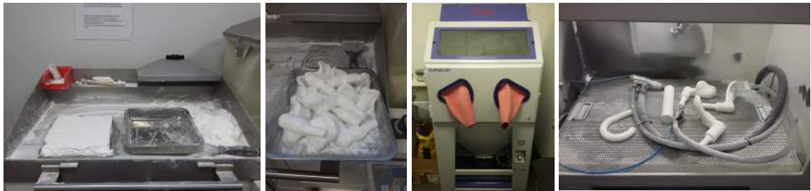
Figure 6.9 - From left to right, parts extracted, Euroblast machine and its inner chamber
