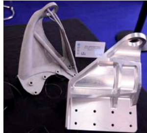
Figure 2.13 - 3D printed optimised aircraft part and original machined part (Boeing and Hamburg University of Technology) [74]
