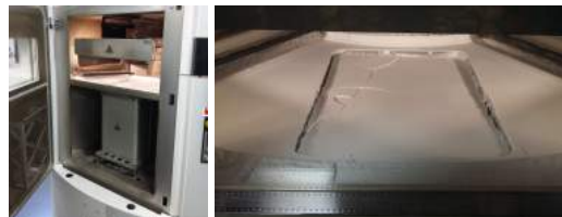
Figure 6.8 - EOS Formiga P100 laser sintering machine and the inner build chamber
