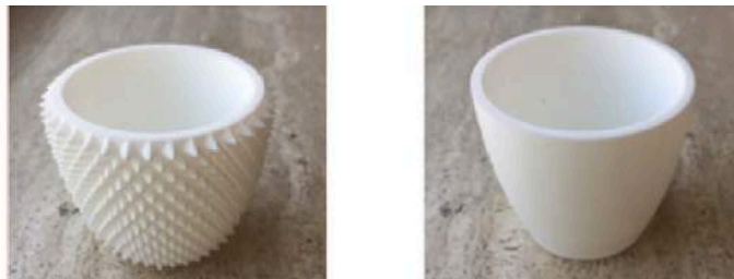
Figure 6.2 - Cup with sharp texture surface (left) and smooth texture surface (right) [197]
