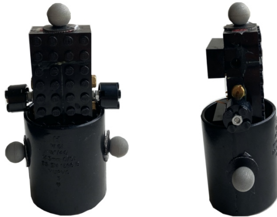
Figure 4.1: The initial manipulandum design (Prototype 1) face-on (left) and side-on (right). Two circular plungers, with a small diameter, extend out of the manipulanda body encouraging a precision grip. Additional mass can be attached to the manipulanda via a screw thread under the plastic tube located beneath the grip plungers.
