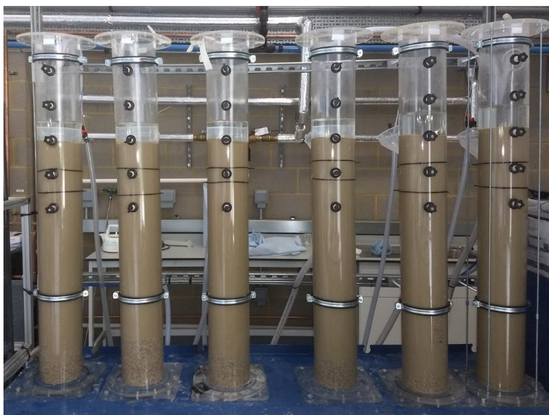
Figure 4-1. Pilot-scale slow sand filters: each filter had a total volume of 22.8 L and a calculated water volume of 6.325 L. Sampling ports were located at different depths throughout the filter.
