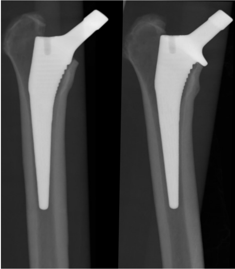
Figure 7-1 Reformatted CT demonstrating anteroposterior view of specimens immediately after implantation with a Corail femoral stem.
