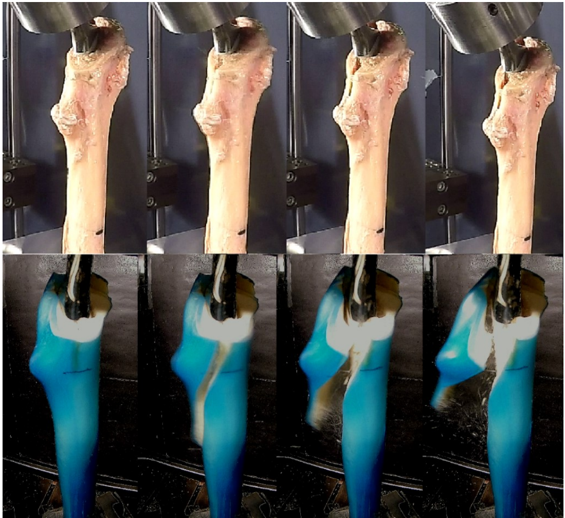
Figure 7-7 Comparison of collarless fracture pattern between human cadaveric specimens (top row) and osteoporotic sawbones (bottom row). Fracture occur in a similar position on the proximal femur. Fracture fragment acceleration is noticeably less in the cadaveric versus composite models.
