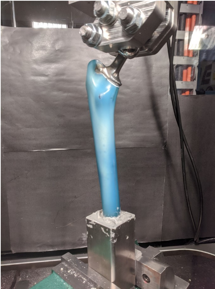
Figure 7-6 Experimental set up for simulated POPFF testing using a composite 'osteoporotic' femur.
