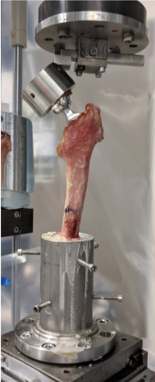
Figure 7-2 Experimental set up in the materials testing machine prior to fracture protocol.
