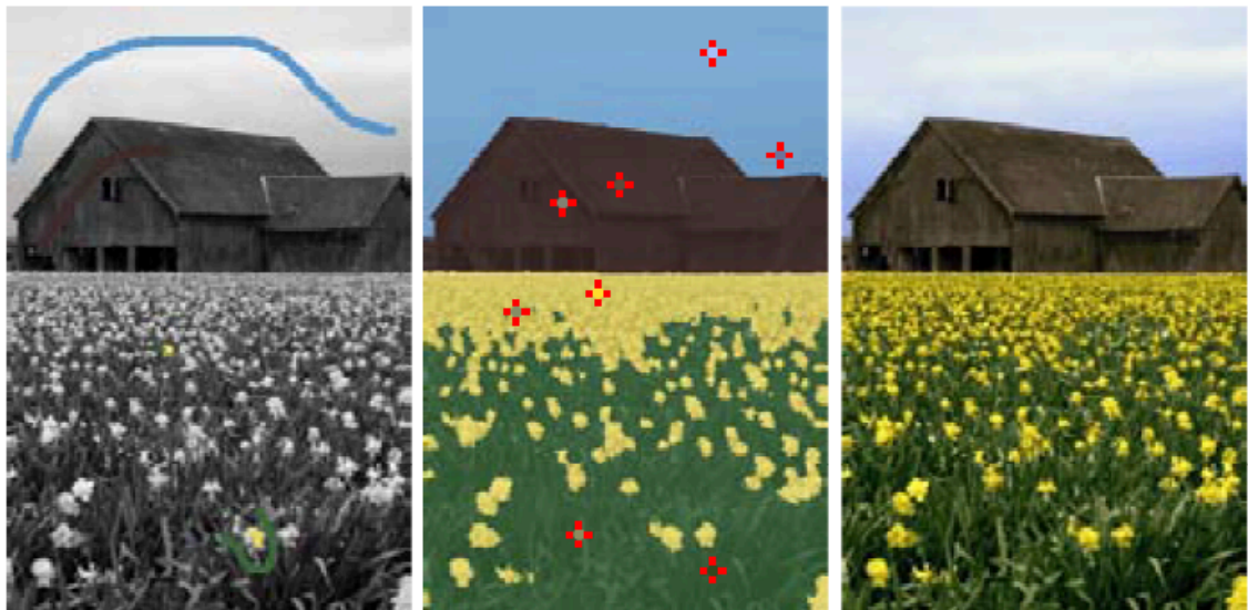
Figure 2-24 Illustration of the colourisation process, scribbling strokes (left), then colour mapping (middle), final colourisation result (right)
