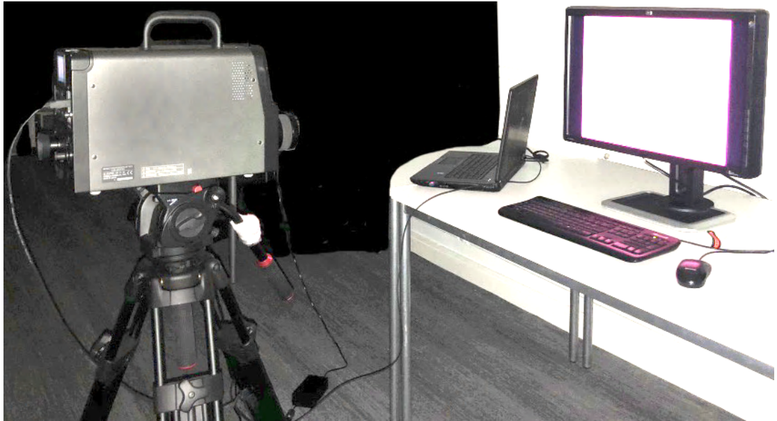
Figure 3-7 Colour measurement of using the Konica Minolta CS-2000.
