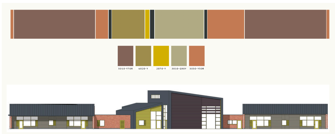
Figure 2-28 Buildings for Colwall Primary School drawn from detailed manual extracted colour palette from local landscape (Waygood, 2017).
