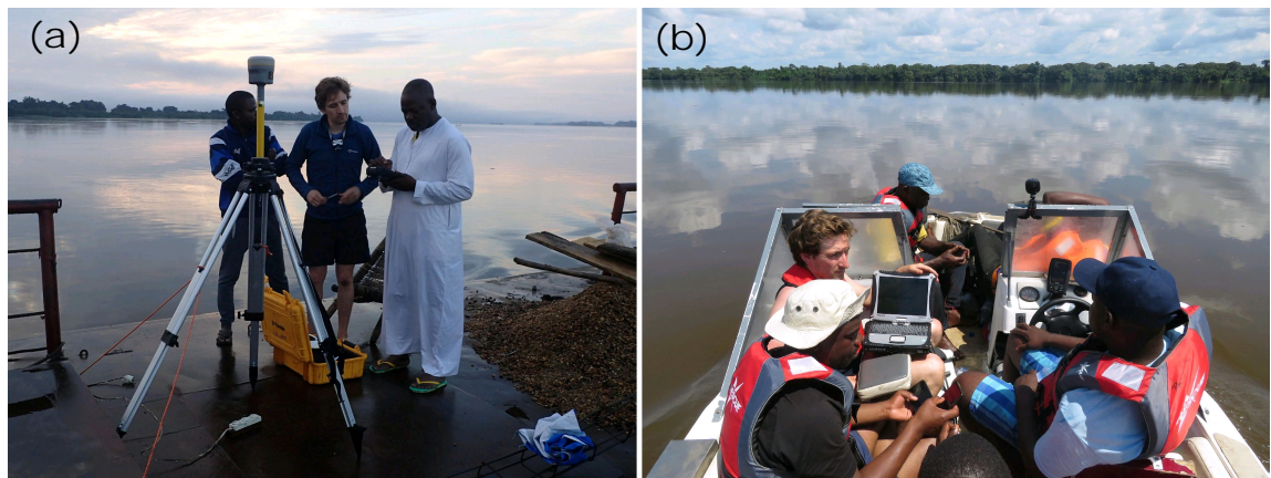
Fig. A-2. Fieldwork measurements: (a) early morning setup of GNSS; (b) Conducting an ADCP transect.
