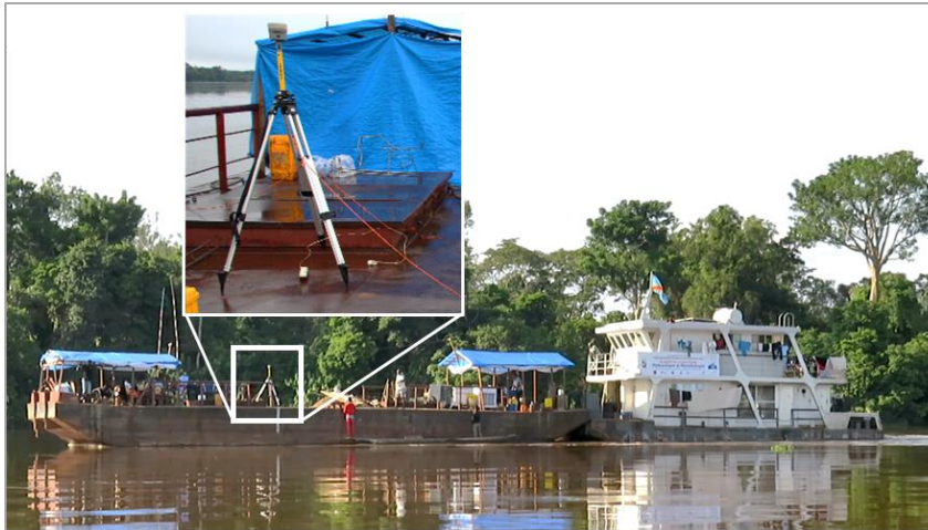
Figure 4-9. GNSS instrument set up on the barge being pushed by the main boat, for continuous WSE measurements on 2019 field campaign.
