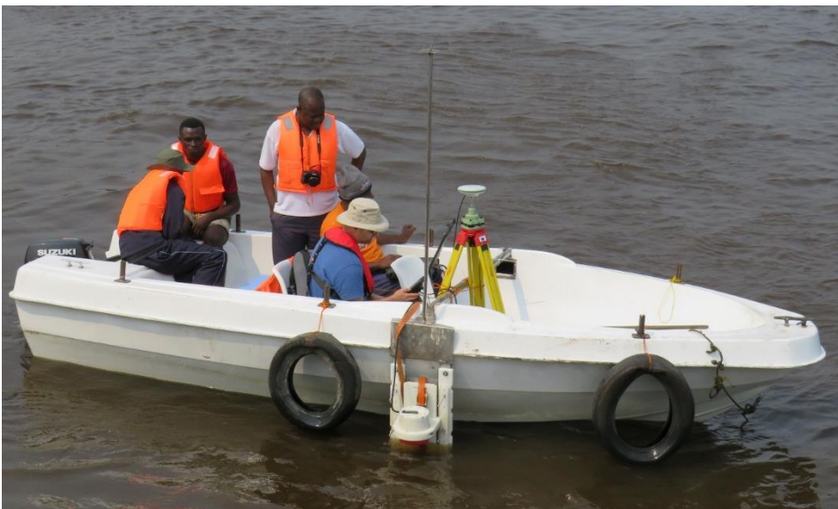
Figure 4-3. ADCP fixed in place on the side of the fibreglass boat, prior to being fully lowered into the water.
