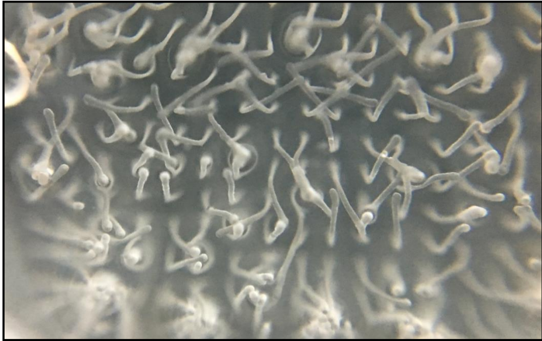
Figure 71 Paraffin wax microstructures encapsulated in PDMS
