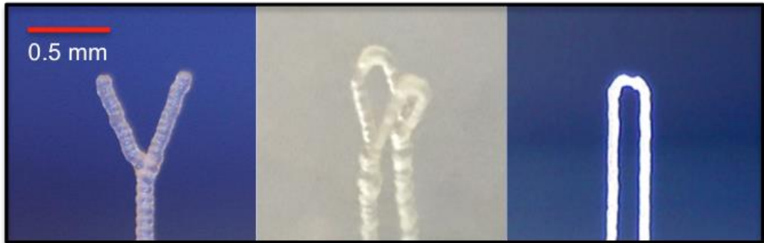
Figure 49 Two 30-layer multi-droplet columns, positioned with 300 micron between column' centres, supporting four 15-droplet angled columns. Multi-droplet columns consist of 30 layers of 2 droplets, deposited in a burst at 1024 Hz, with an effective delay between droplet bursts of 0.25 s. Angled columns: consist of 15 droplets deposited in accordance with the speed of the substrate movement (moving in 10 micron increments per deposited droplet from the point of bifurcation). Arch: decrease gap between the uppermost point of each column from 300 micron to 30 micron, in increments of 10 - 20-micron, then add 'keystone'.
