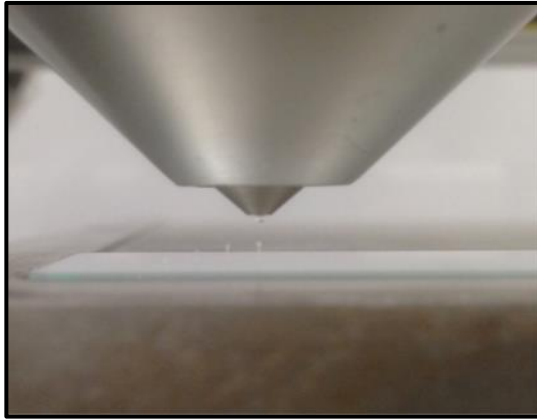
Figure 14 The thermal mass of the high temperature printhead.
