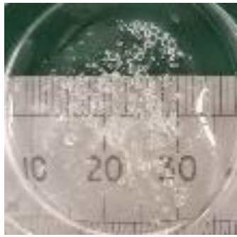
Figure 2.13 Dissolution of C2-20 after 24-hour immersion in the simulated wound fluid containing 20 mM GSH. The material was too fragile to undergo any form of analysis.
