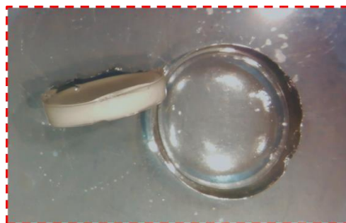
Figure 3.19 Optical images of the wet mineralised sample C2-40 after \text{HPO}_4^{2-} treatment (side view, left) and C2-40 control (top surface, right).
